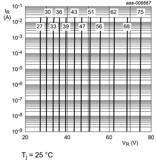
**Fig. 10.** Reverse current as a function of reverse voltage; typical values (BZX84-A/B/C27-Q to BZX84-A/B/C75-Q)
