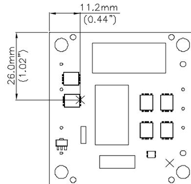
Figure 21: Temperature measurement location
