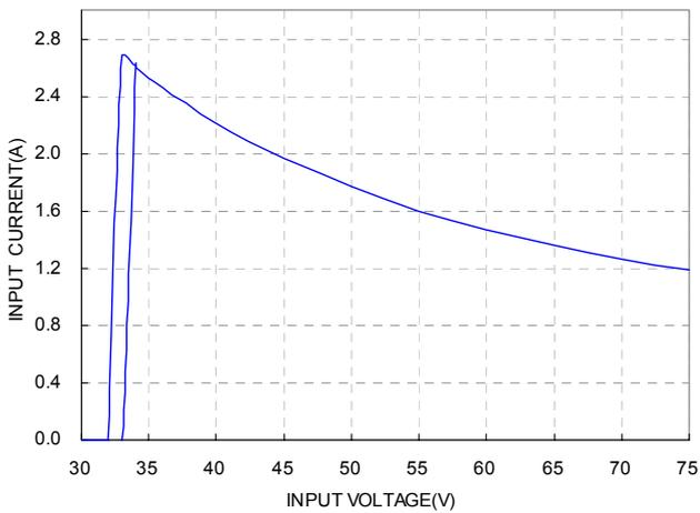
**Figure 3:** Typical input characteristics at room temperature
