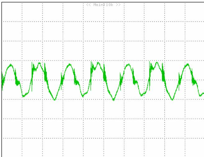
**Figure 14:** Output voltage ripple at nominal input voltage and rated load current ( $10\text{mV/div}$ ). Load capacitance:  $1\mu\text{F}$  ceramic capacitor and  $10\mu\text{F}$  Flow ESR capacitor. Bandwidth:  $20\text{MHz}$ . Scope measurement should be made using a BNC cable (length shorter than 20 inches). Position the load between 51 mm to 76 mm (2 inches to 3 inches) from the module.
