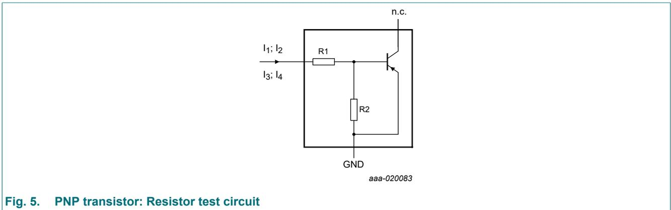
Fig. 5. PNP transistor: Resistor test circuit
