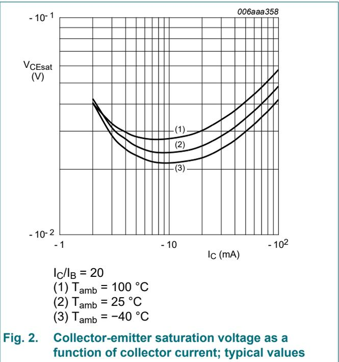
50 V, 500 mA PNP resistor-equipped transistor; R1 = 2.2 kΩ, R2 = 10 kΩ
