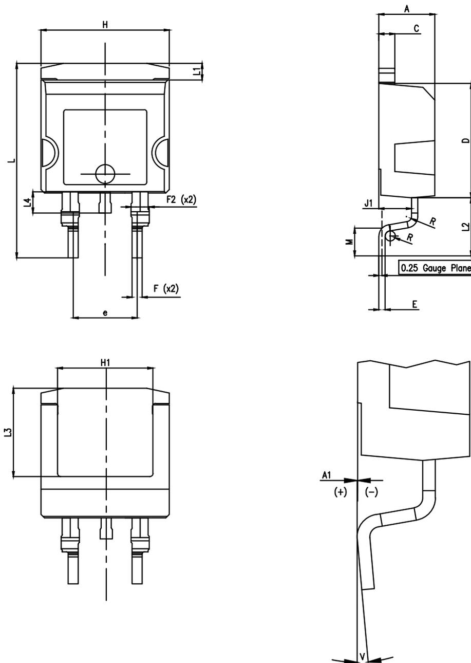
**Table 5. D<sup>2</sup>PAK high voltage package mechanical data**
