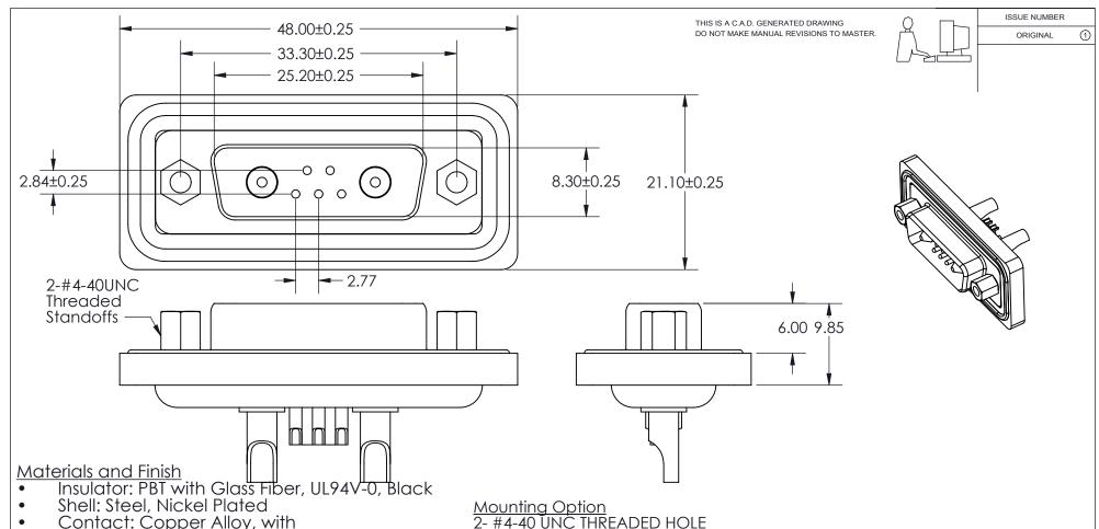
Contact: Copper Alloy, with 2-Gold Flash Plating over Nickel Watertight Frame: PBT with Glass Fiber, UL94V-0,
