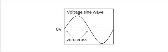
\*ZERO CROSS is the point where voltage sine wave passes 0V. See the figure at right.
