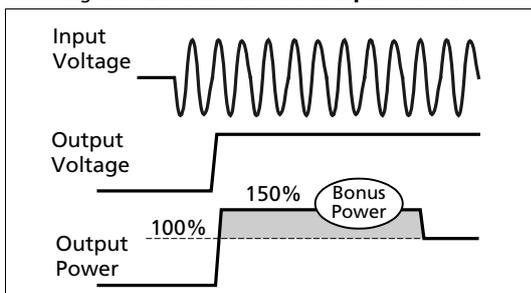
Fig. 6-8 BonusPower<sup>®</sup> after output short
