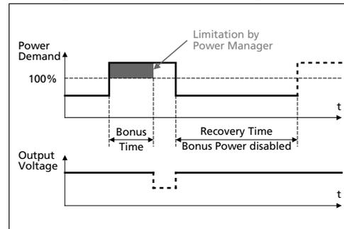
The BonusPower<sup>®</sup> is available as soon as power comes on and after the end of an output short circuit or output overload.
