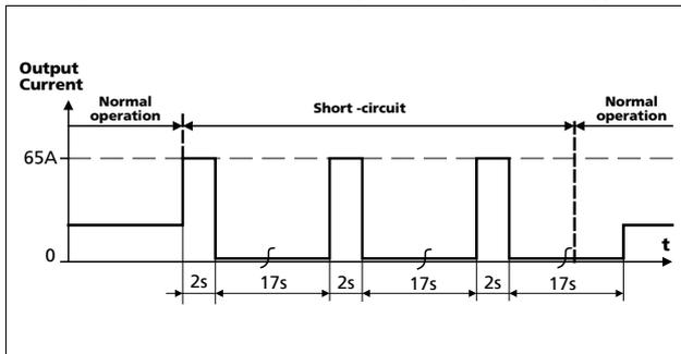
Fig. 6-4 Dynamic overcurrent capability, typ.
