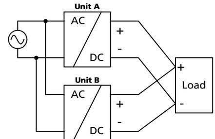
If more than three units are connected in parallel, a fuse or circuit breaker with a rating of 50A or 63A is required on each output. Alternatively, a diode or redundancy module can also be utilized.
