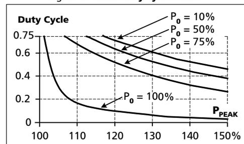
$$\text{DutyCycle} = \frac{T_{\text{peak}}}{T_{\text{peak}} + T_0}$$
