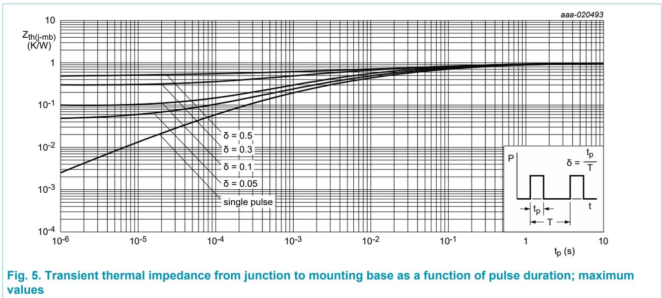
Fig. 5. Transient thermal impedance from junction to mounting base as a function of pulse duration; maximum values
