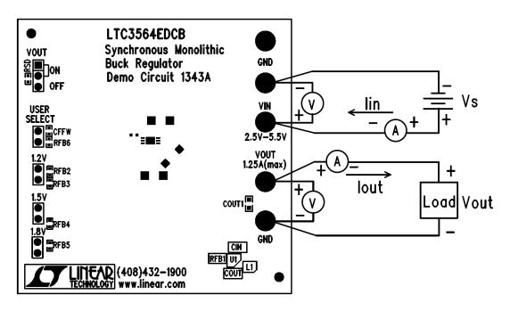
Figure 2. Proper Measurement Equipment Setup
