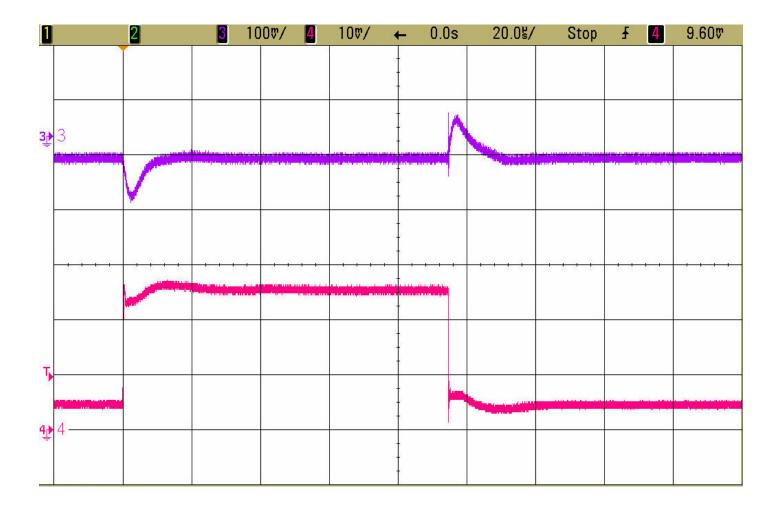
Figure 3. Load Step Response
