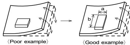
(2) Components location on PCB separation
