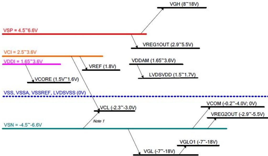
Figure 130: Power Structure of Power Mode 4
