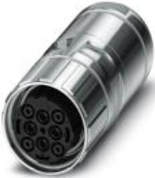
Cable connector, straight long, Screw locking, M40, Number of positions: 4+3+PE, Type of contact: Socket, Crimp connection, Shielded: Yes, Cable cross section: 20.5 mm...26.5 mm
