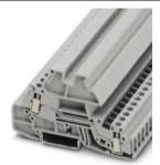
Installation level terminal block, Screw connection, Cross section: 0.2 mm² - 4 mm², AWG: 24 - 12, Width: 6.2 mm, Color: gray, Mounting type: NS 35/7,5, NS 35/15
