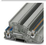
Installation level terminal block, Push-in connection, Cross section: 0.14 mm² - 4 mm², AWG: 26 - 12, Width: 5.2 mm, Color: gray/blue, Mounting type: NS 35/7,5, NS 35/15
