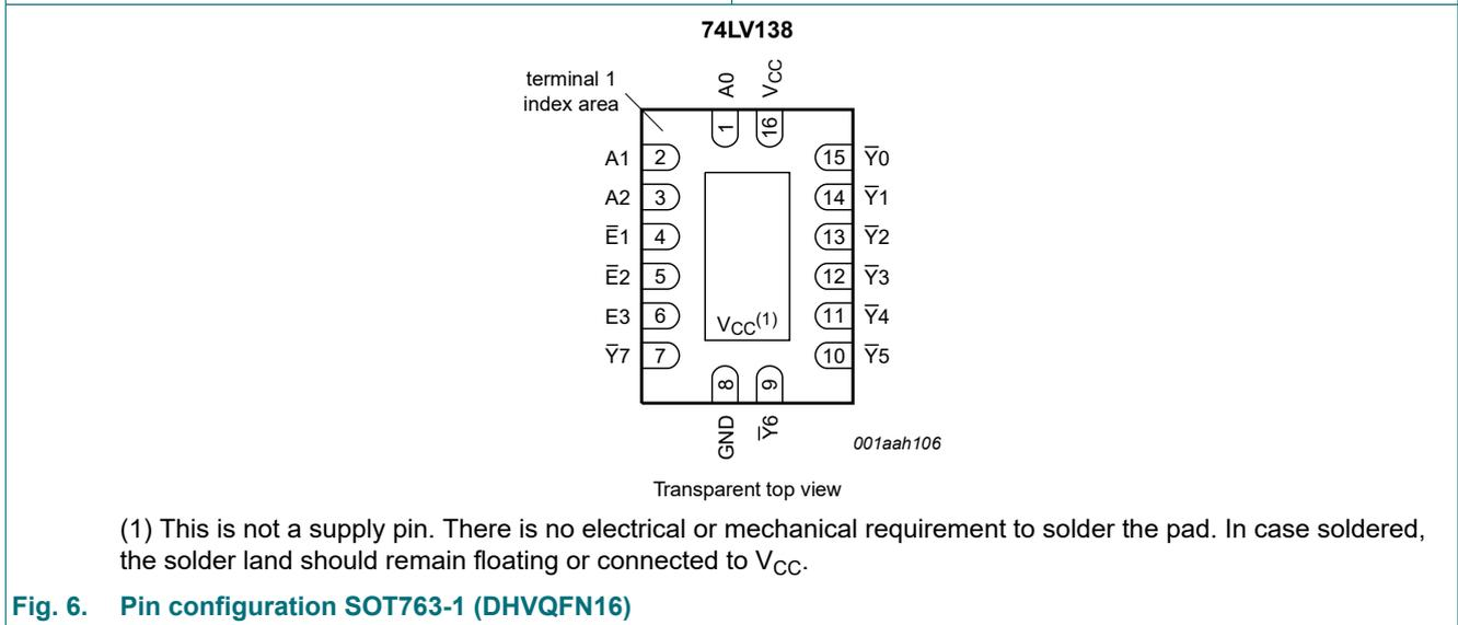
Fig. 6. Pin configuration SOT763-1 (DHVQFN16)
