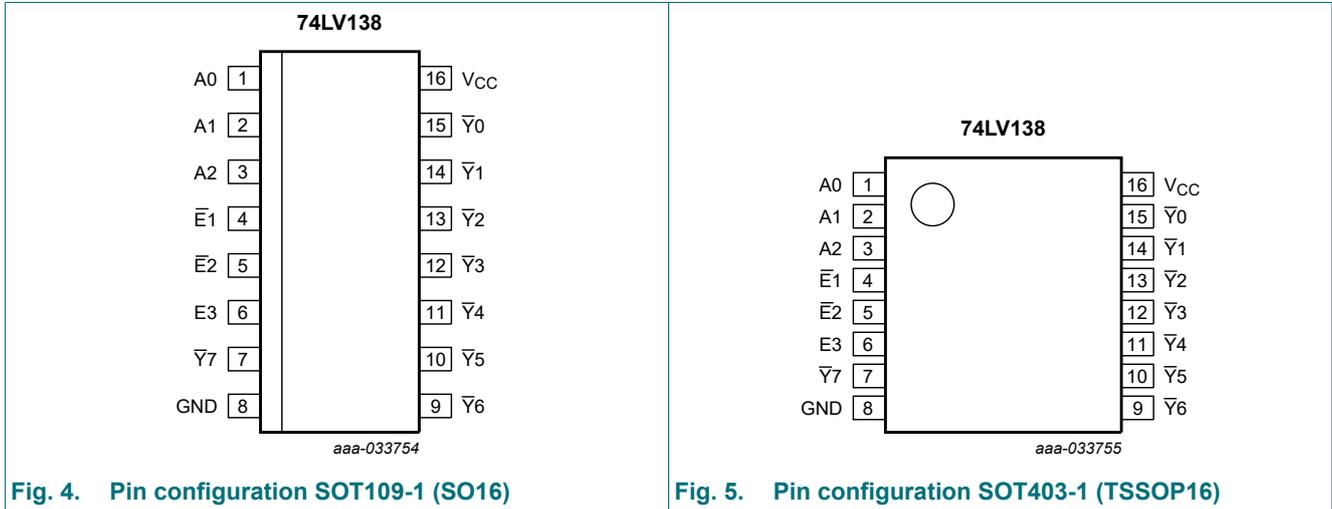
Fig. 4. Pin configuration SOT109-1 (SO16)
