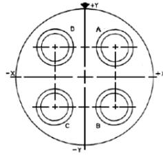
(Inactive for new design for MIL-DTL-38999. For new design, use arrangement no. 21-76.)
