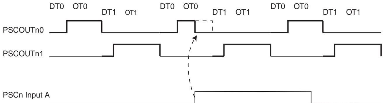
The output frequency is not modified by the occurrence of significant edge of retriggering input.
