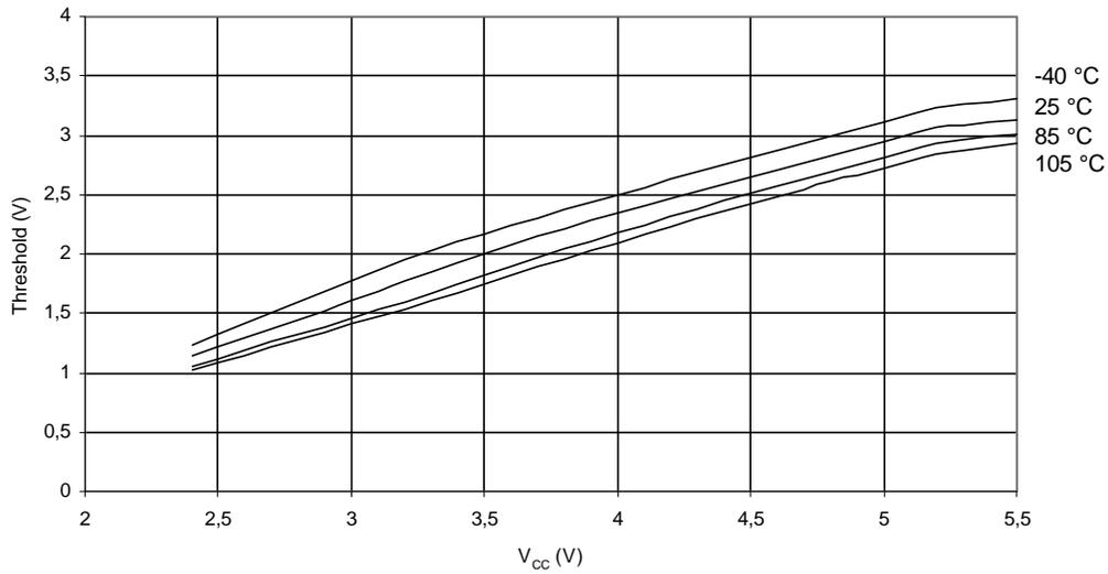
**Figure 26-27.** XTAL1 Input Threshold Voltage vs.  $V_{CC}$  (XTAL1 Pin Read As '0')
