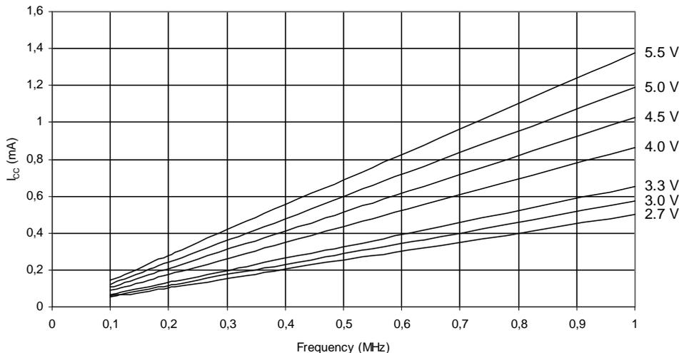
**Figure 26-2.** Active Supply Current vs. Frequency (1 - 24 MHz)
