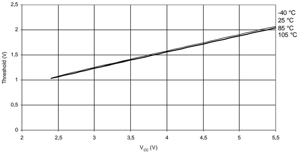
**Figure 26-21. I/O Pin Input Threshold Voltage vs.  $V_{CC}$  (VIL, I/O Pin Read As '0')**
