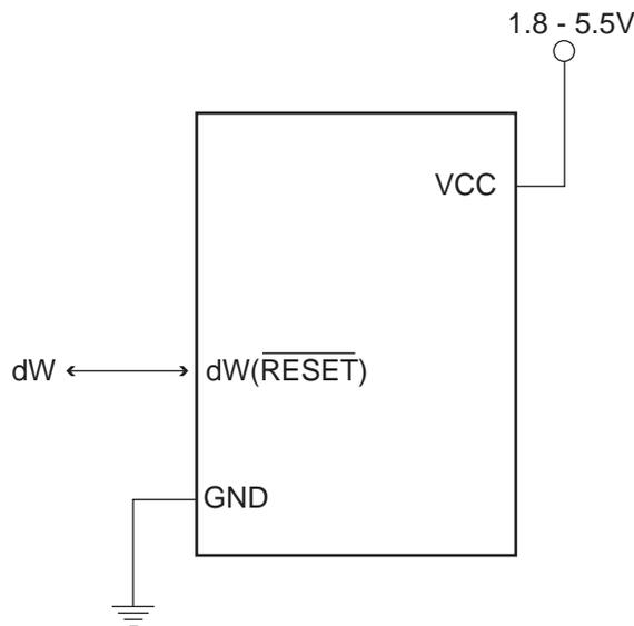
Figure 22-1 shows the schematic of a target MCU, with debugWIRE enabled, and the emulator connector. The system clock is not affected by debugWIRE and will always be the clock source selected by the CKSEL Fuses.
