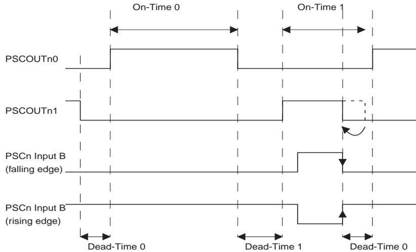
Note: This example is given in “Input Mode 8” in “2 or 4 ramp mode” See Figure 15-31. for details.
