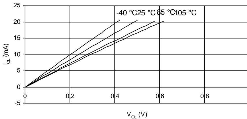
**Figure 26-19.** I/O Pin Sink Current vs. Output Voltage ( $V_{CC} = 2.7V$ )
