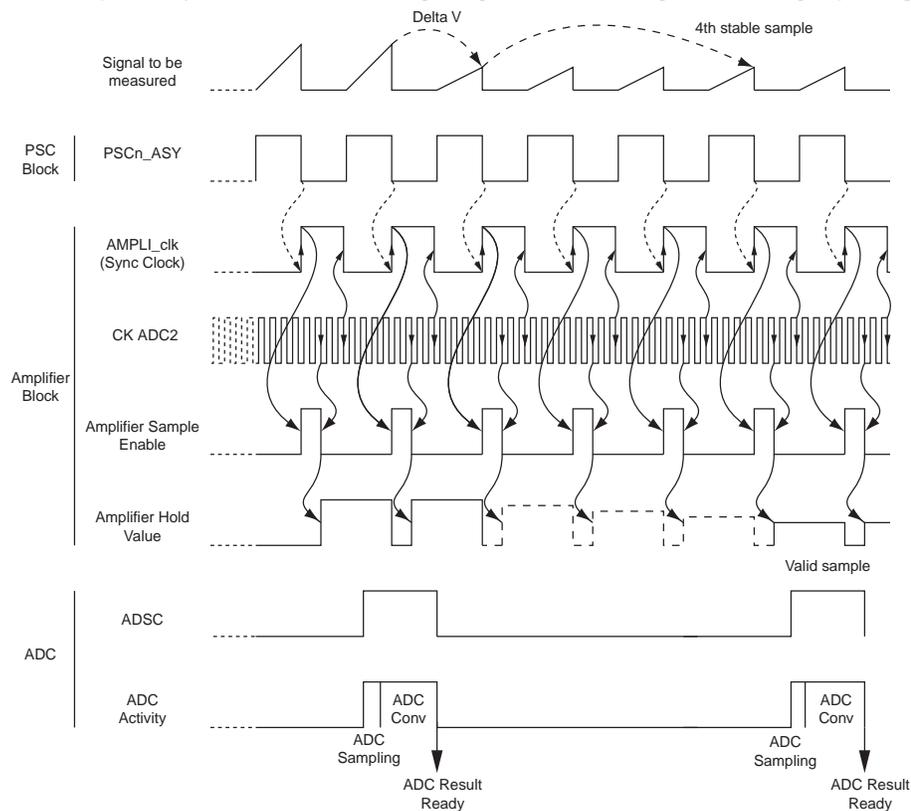
**Figure 20-16.** Amplifier synchronization timing diagram: behavior when ADSC is set when the amplifier output is changing.
