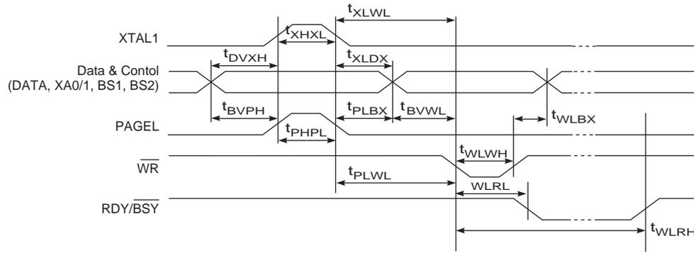
**Figure 24-8.** Parallel Programming Timing, Loading Sequence with Timing Requirements<sup>(1)</sup>
