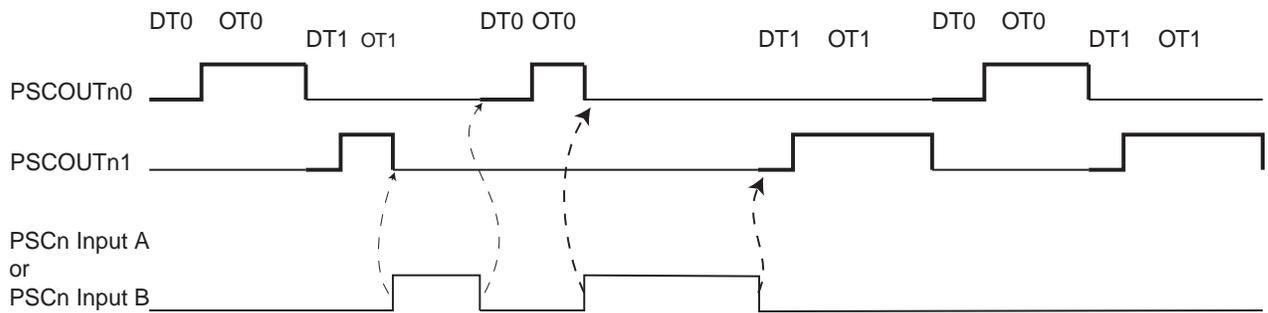
Used in Fault mode 6, PSCn Input A or PSCn Input B act indifferently on On-Time0/Dead-Time0 or on On-Time1/Dead-Time1.
