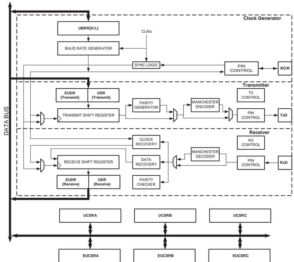
The EUSART is activated with the EUSART bit of EUCSRB register. Until this bit is not set, the USART will behave as standard USART, all the functionalities of the EUSART are not accessible.
