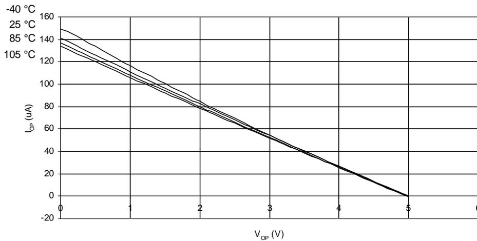
**Figure 26-13. I/O Pin Pull-Up Resistor Current vs. Input Voltage ( $V_{CC} = 2.7V$ )**
