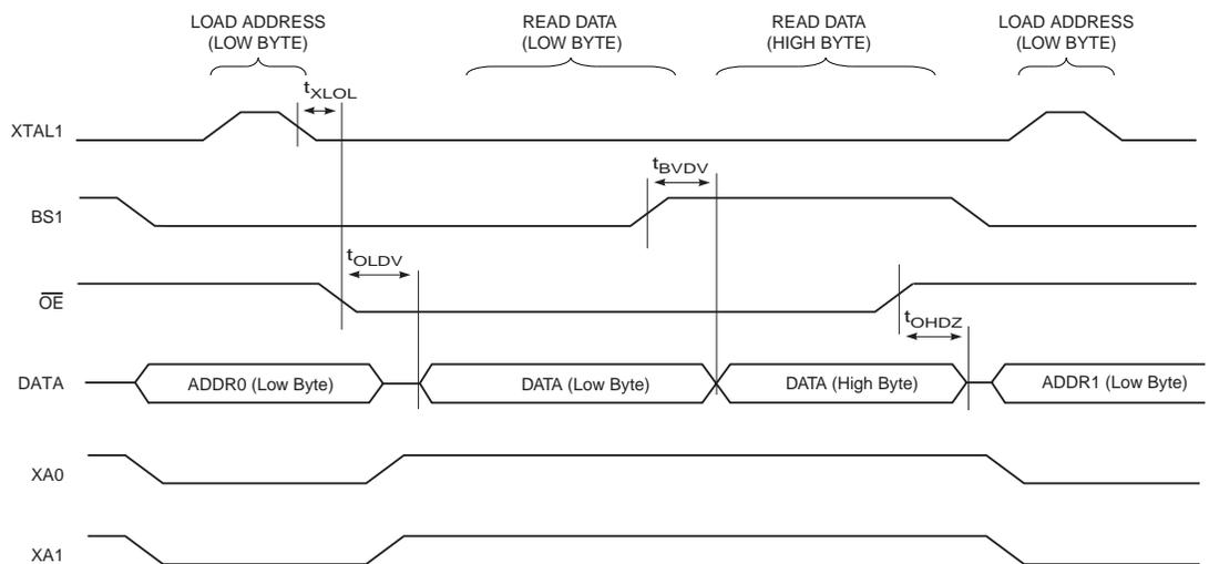
Note: 1. The timing requirements shown in Figure 25-5 (i.e.,  $t_{DVXH}$ ,  $t_{XHXL}$ , and  $t_{XLDX}$ ) also apply to reading operation.
