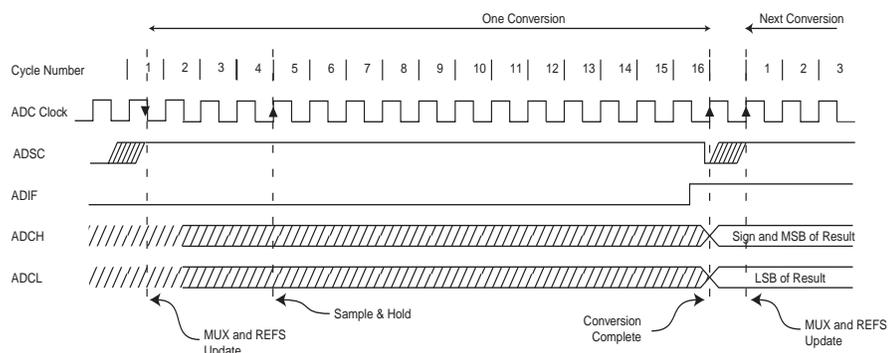
**Figure 20-6.** ADC Timing Diagram, Auto Triggered Conversion
