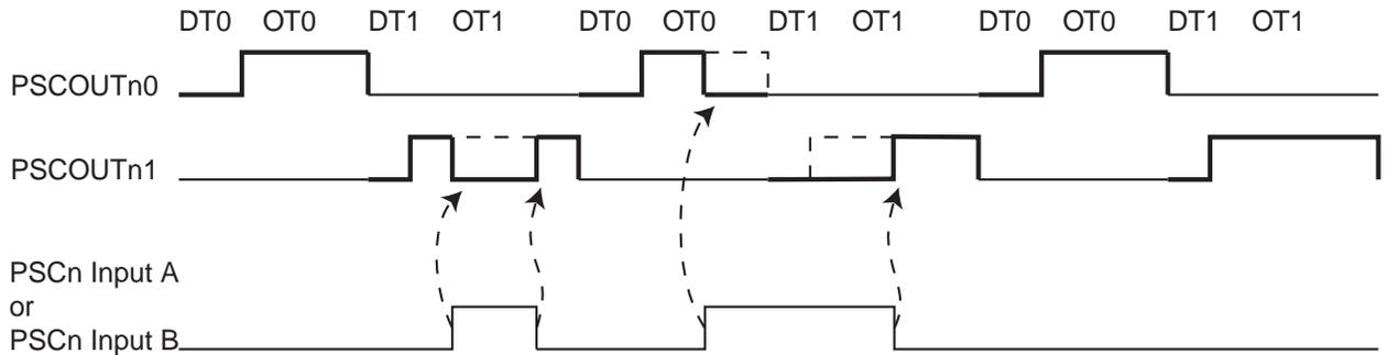
**Figure 15-27.** PSC behaviour versus PSCn Input A or Input B in Fault Mode 4
