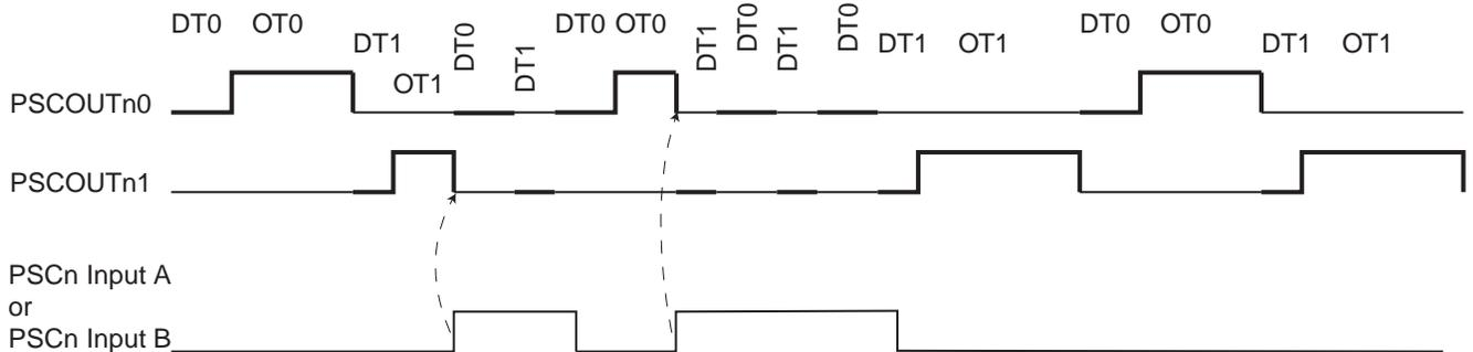
Used in Fault mode 5, PSCn Input A or PSCn Input B act indifferently on On-Time0/Dead-Time0 or on On-Time1/Dead-Time1.
