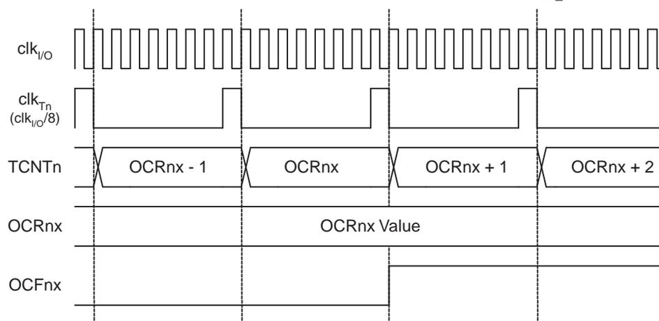
[Figure 14-12](#) shows the count sequence close to TOP in various modes. When using phase and frequency correct PWM mode the OCRnx Register is updated at BOTTOM. The timing diagrams will be the same, but TOP should be replaced by BOTTOM, TOP-1 by BOTTOM+1 and so on. The same renaming applies for modes that set the TOVn Flag at BOTTOM.
