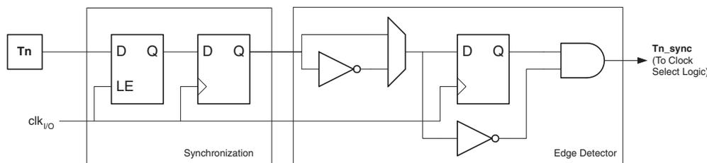
The synchronization and edge detector logic introduces a delay of 2.5 to 3.5 system clock cycles from an edge has been applied to the Tn/T0 pin to the counter is updated.
