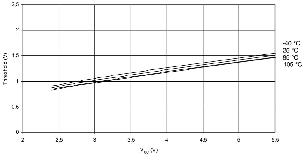
**Figure 26-22. I/O Pin Input Hysteresis Voltage vs.  $V_{CC}$**
