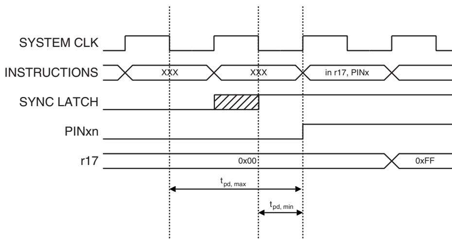
Consider the clock period starting shortly after the first falling edge of the system clock. The latch is closed when the clock is low, and goes transparent when the clock is high, as indicated by the shaded region of the “SYNC LATCH” signal. The signal value is latched when the system clock goes low. It is clocked into the PINx<sub>n</sub> Register at
