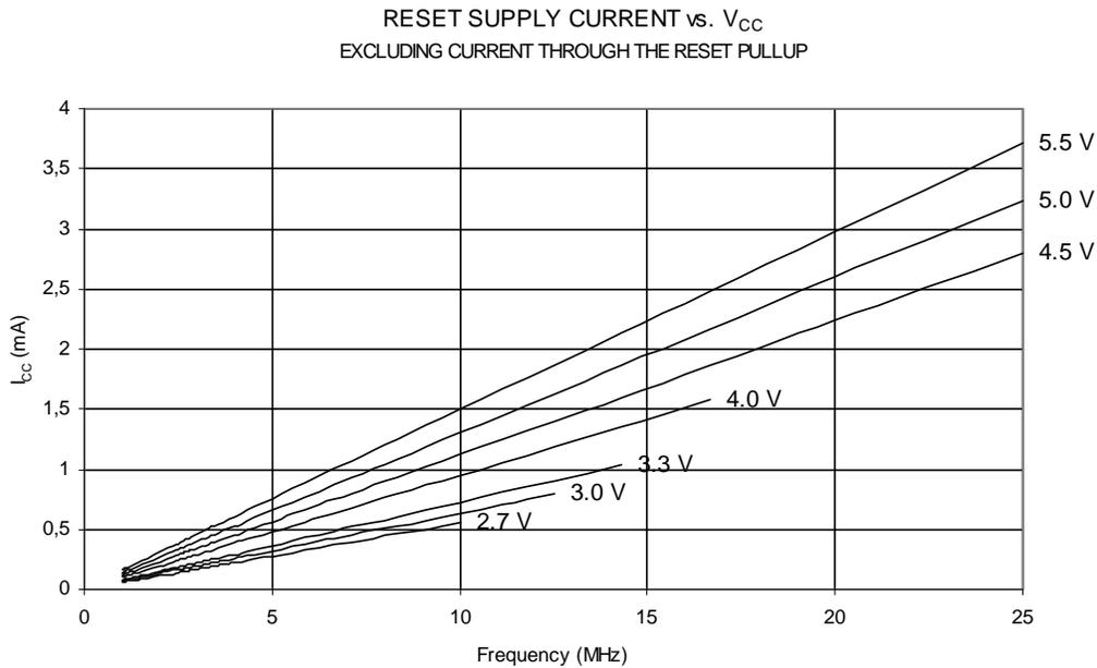
**Figure 26-47. Reset Supply Current vs.  $V_{CC}$  (Clock Stopped, Excluding Current through the Reset Pull-up)**
