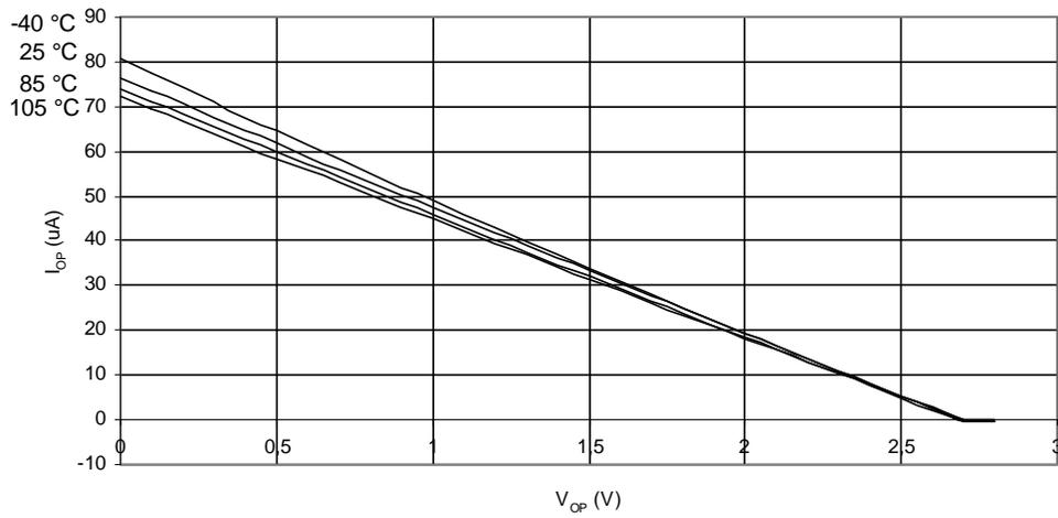
**Figure 26-14. Reset Pull-Up Resistor Current vs. Reset Pin Voltage ( $V_{CC} = 5V$ )**
