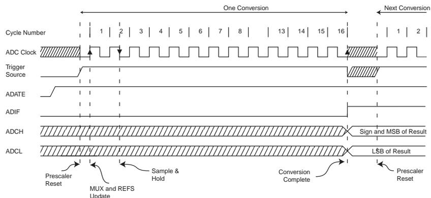
**Figure 20-7.** ADC Timing Diagram, Free Running Conversion
