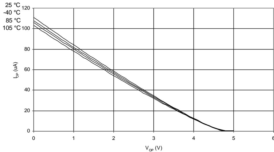
**Figure 26-15. Reset Pull-Up Resistor Current vs. Reset Pin Voltage ( $V_{CC} = 2.7V$ )**
