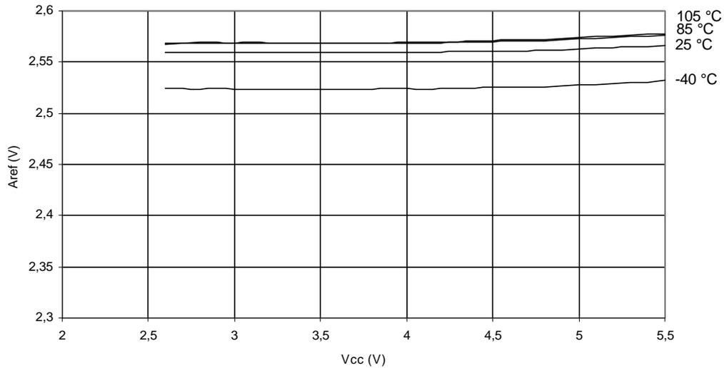
**Figure 26-35.** AREF Voltage vs. Temperature
