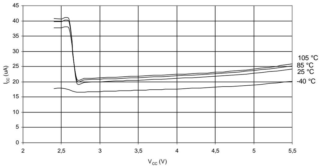
**Figure 26-41.** ADC Current vs.  $V_{CC}$  (ADC at 50 kHz)
