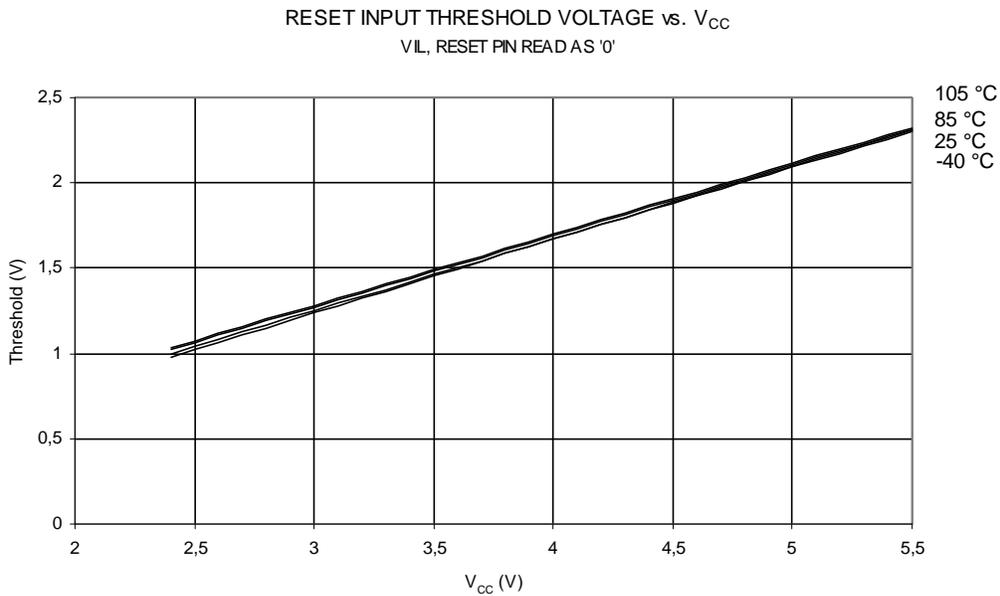
**Figure 26-25.** Reset Input Pin Hysteresis vs.  $V_{CC}$
