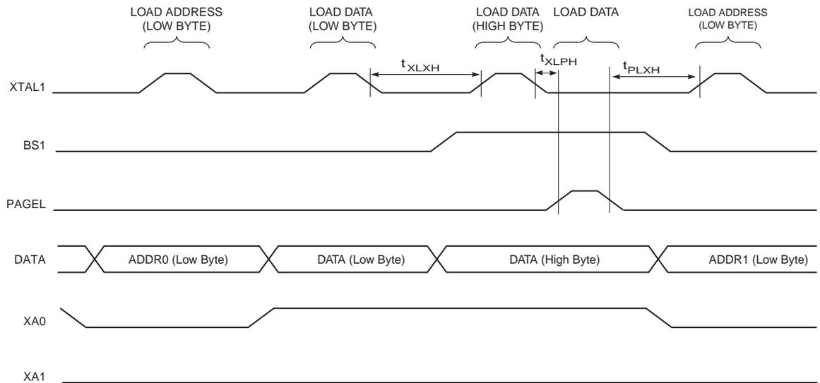
Note: 1. The timing requirements shown in Figure 25-5 (i.e.,  $t_{DVXH}$ ,  $t_{XHXL}$ , and  $t_{XLDX}$ ) also apply to loading operation.
