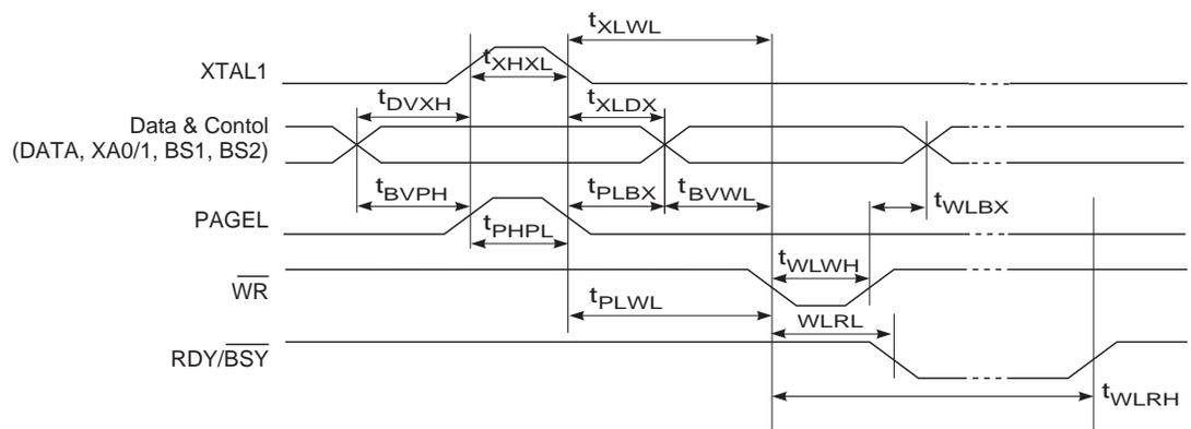
**Figure 25-6.** Parallel Programming Timing, Loading Sequence with Timing Requirements<sup>(1)</sup>
