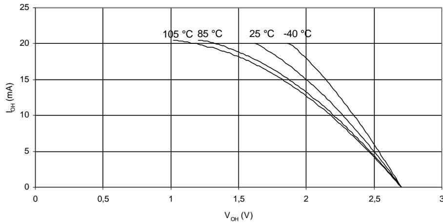
**Figure 26-18.** I/O Pin Sink Current vs. Output Voltage ( $V_{CC} = 5V$ )
