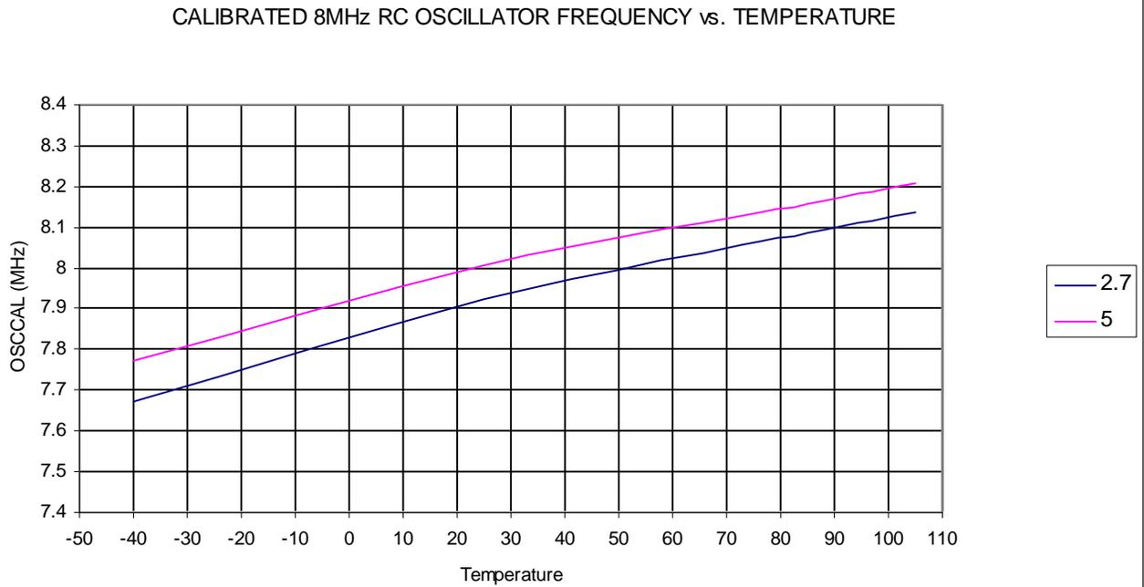
**Figure 26-38.** Calibrated 8 MHz RC Oscillator Frequency vs.  $V_{CC}$
