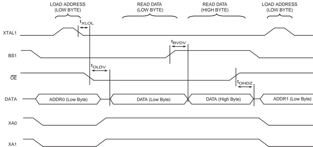
Note: 1. The timing requirements shown in Figure 24-7 (i.e.,  $t_{DVXH}$ ,  $t_{XHXL}$ , and  $t_{XLDX}$ ) also apply to reading operation.
