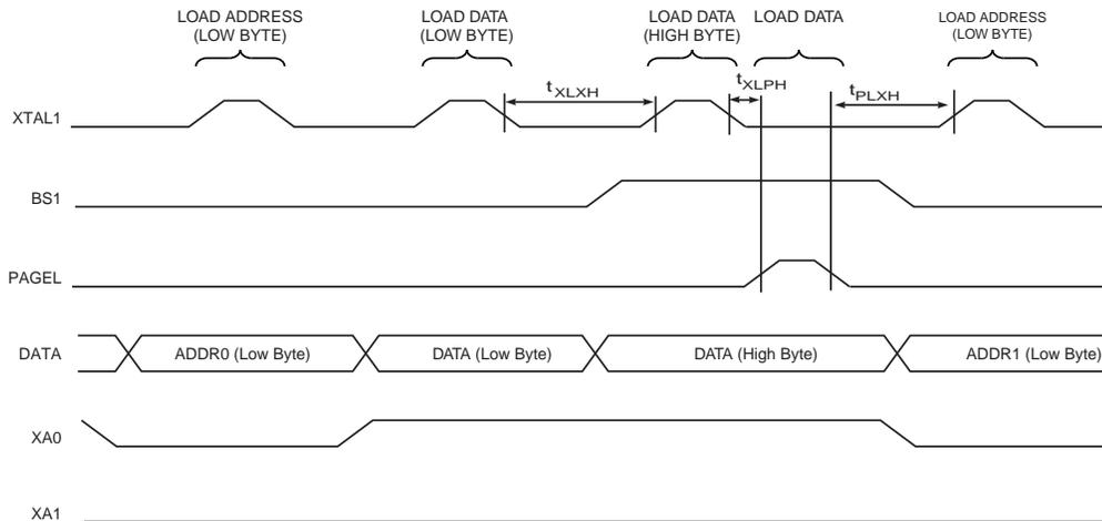
Note: 1. The timing requirements shown in [Figure 24-7](#) (i.e.,  $t_{DVXH}$ ,  $t_{XHXL}$ , and  $t_{XLDX}$ ) also apply to loading operation.
