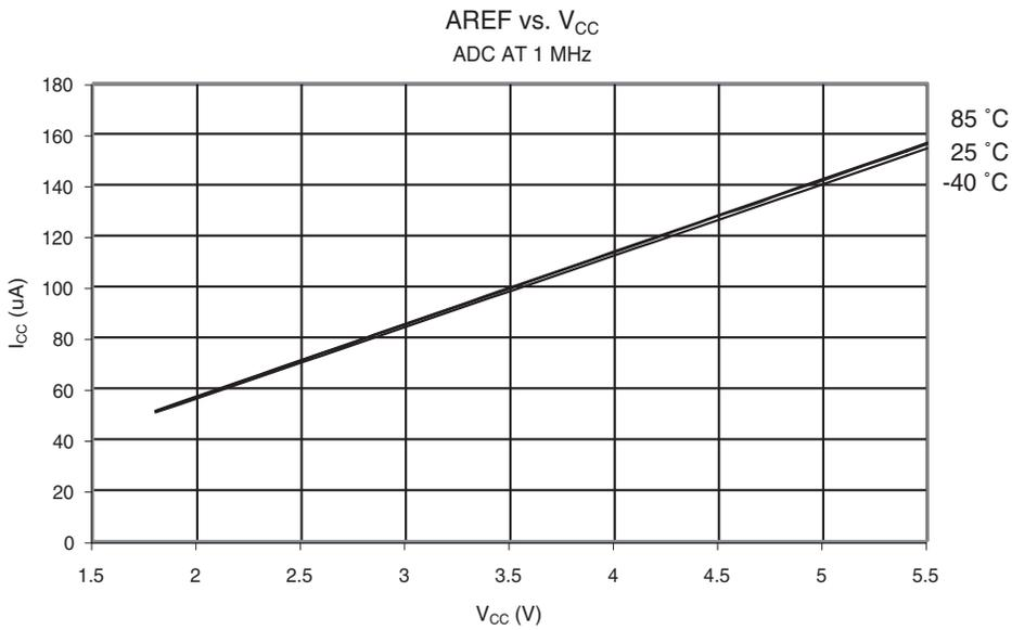
**Figure 26-43.** Analog Comparator Current vs.  $V_{CC}$
