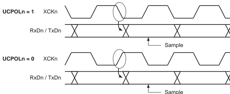
The UCPOL bit UCRSnC selects which XCK clock edge is used for data sampling and which is used for data change. As [Figure 17-3](#) shows, when UCPOL is zero the data will be changed at rising XCK edge and sampled at falling XCK edge. If UCPOL is set, the data will be changed at falling XCK edge and sampled at rising XCK edge.
