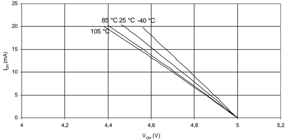
**Figure 26-17.** I/O Pin Source Current vs. Output Voltage ( $V_{CC} = 2.7V$ )
