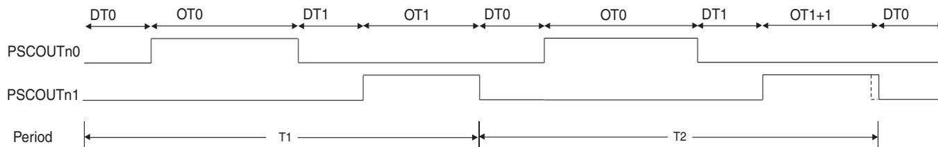
The supplementary step in counting to generate  $f_{b2}$  is added on the PSCn0 signal while needed in the frame according to the fractional divider. See [Table 15-5, "Distribution of fb2 in the modulated frame," on page 134.](#)
