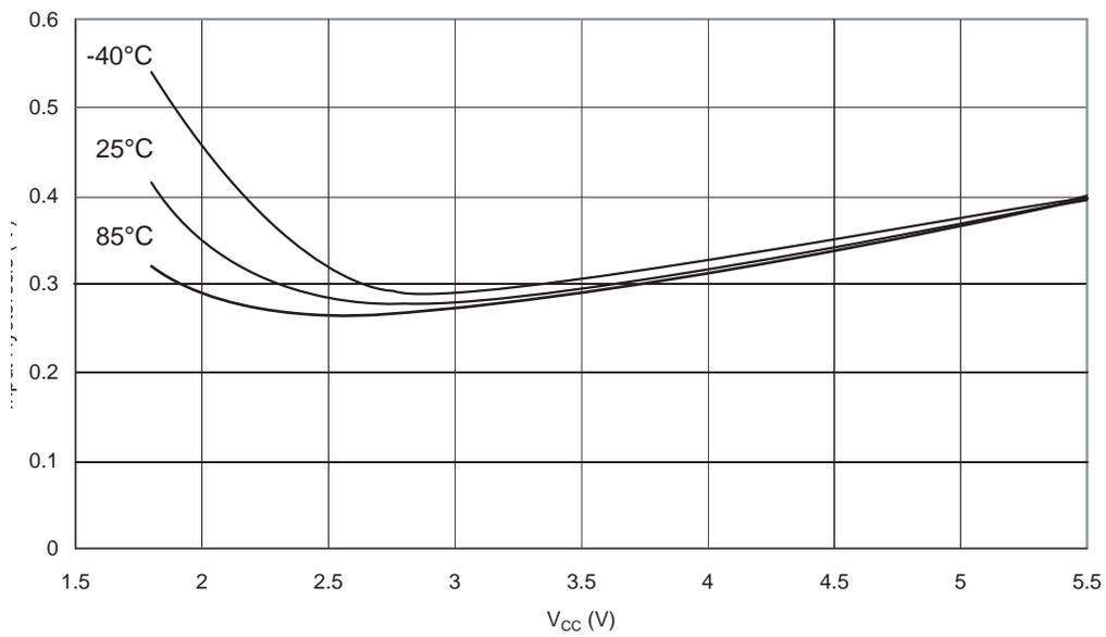
**Figure 26-23.** Reset Input Threshold Voltage vs.  $V_{CC}$  ( $V_{IH}$ , Reset Pin Read As '1')
