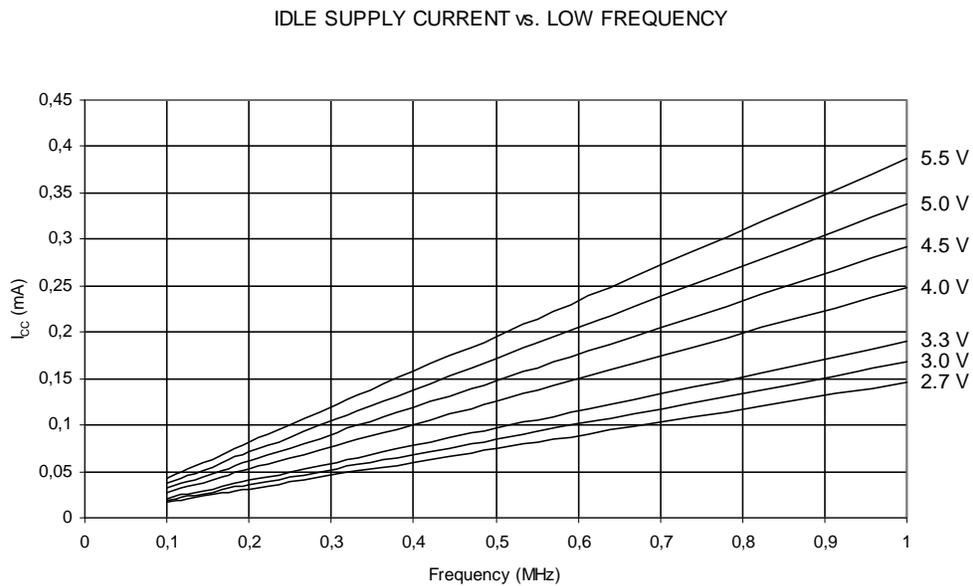
**Figure 26-6.** Idle Supply Current vs. Frequency (1 - 24 MHz)
