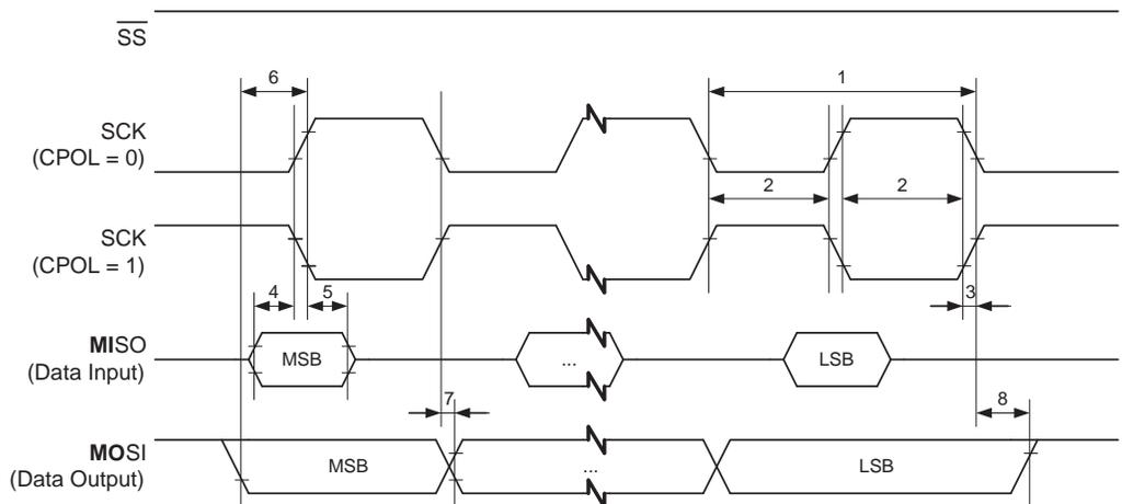
**Figure 25-4.** SPI Interface Timing Requirements (Slave Mode)
