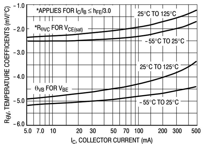
Figure 11. Temperature Coefficients
