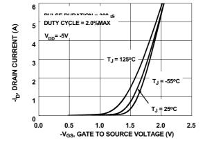
Figure 5. Transfer Characteristics
