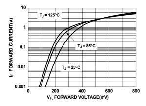
Figure 11. Schottky Diode Forward Voltage
