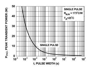
Figure 10. Single Pulse Maximum Power Dissipation
