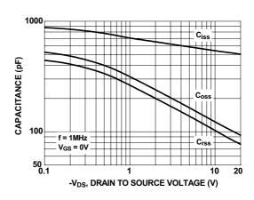
Figure 8. Capacitance Characteristics
