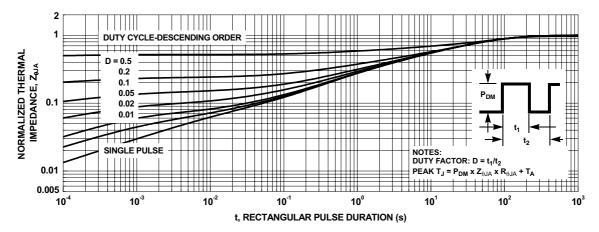
Figure 13. Transient Thermal Response Curve
