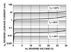
Figure 12. Schottky Diode Reverse Current
