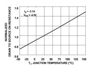
Figure 3. Normalized On-Resistance vs Junction Temperature
