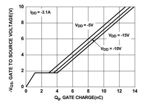
Figure 7. Gate Charge Characteristics
