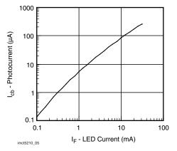
Fig. 6 - Photocurrent vs. LED Current
