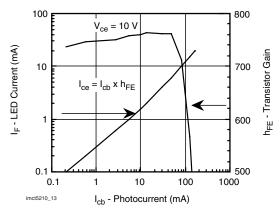
Fig. 13 - Transfer Curve
