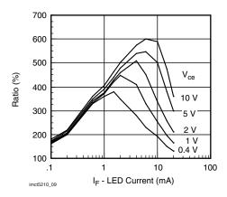
Fig. 9 - CTR vs. LED Current
