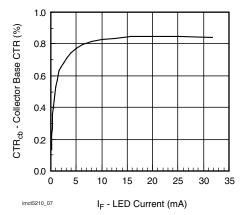
Fig. 7 - Collector Base CTR vs. LED Current
