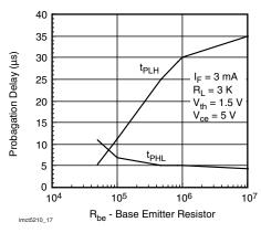
Fig. 17 - Propagation Delay vs. Base Emitter Resistor
