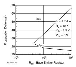
Fig. 15 - Propagation Delay vs. Base Emitter Resistor
