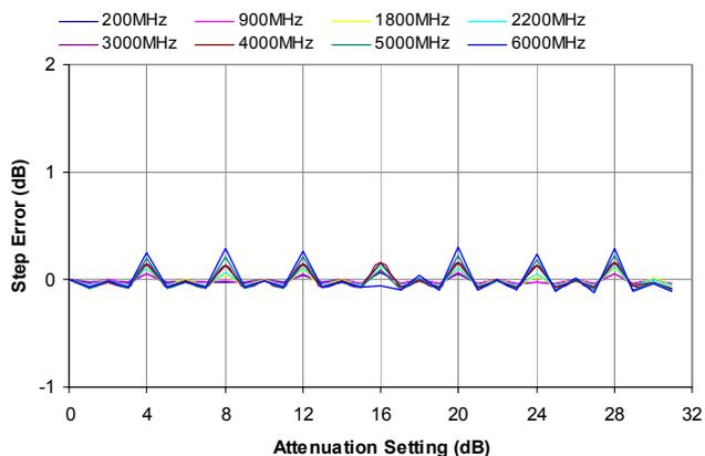
\*Monotonicity is held so long as Step-Error does not cross below -1
