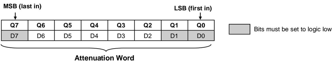
Attenuation Word is derived directly from the attenuation value. For example, to program the 13 dB state:
