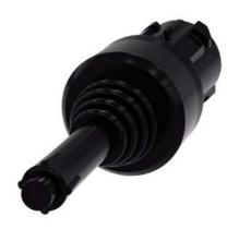
Coordinate switch, 22 mm, round, plastic, black, 2 switch positions, horizontal latching, with mechanical interlocking, with laser labeling, upper case and lower case, always upper case at the beginning of the word
