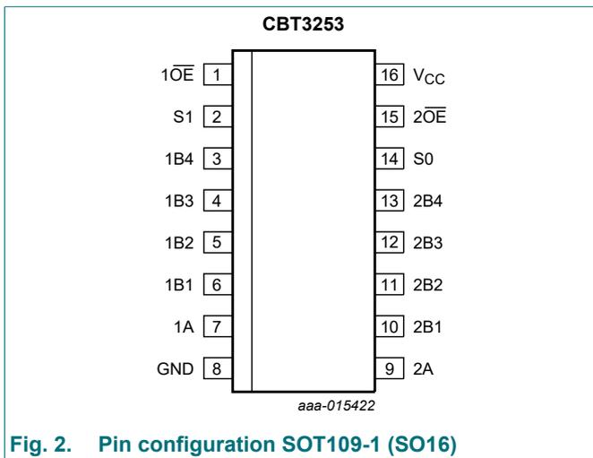
Fig. 2. Pin configuration SOT109-1 (SO16)
