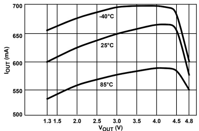
FIGURE 5. CURRENT REGULATION vs V<sub>OUT</sub> (VIN = 5V)
