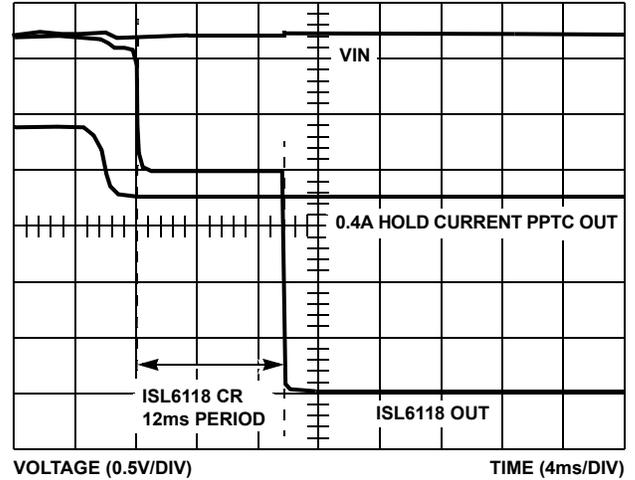
FIGURE 12. ISL6118 vs PPTC INTO 3.5Ω LOAD
