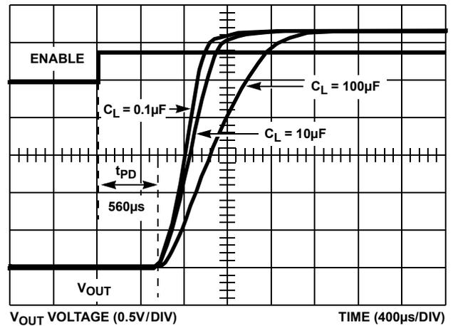
FIGURE 3. V<sub>OUT</sub> SOFT START vs C<sub>L</sub> and PROP DELAY, R<sub>I</sub> = 8Ω
