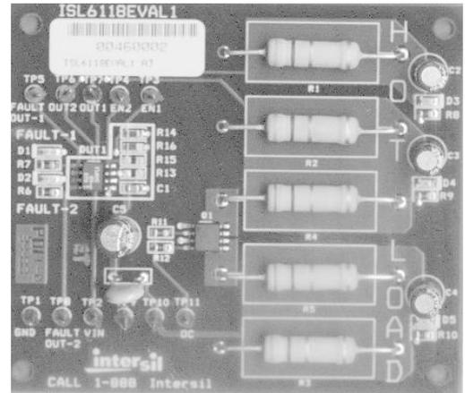
FIGURE 14. ISL6118EVAL1 SCHEMATIC AND PHOTOGRAPH
