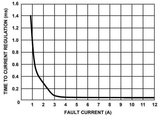
FIGURE 7. CR SETTling TIME vs FAULT CURRENT
