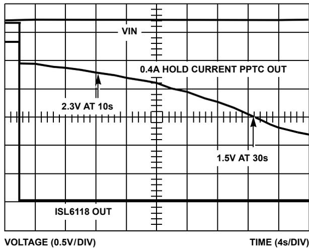
FIGURE 13. ISL6118 vs PPTC WITH EXTENDED 3.5Ω LOAD
