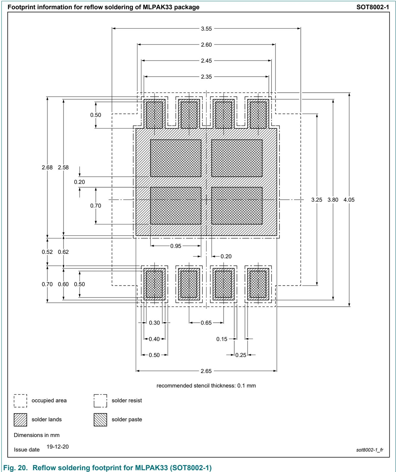
Fig. 20. Reflow soldering footprint for MLPAK33 (SOT8002-1)
