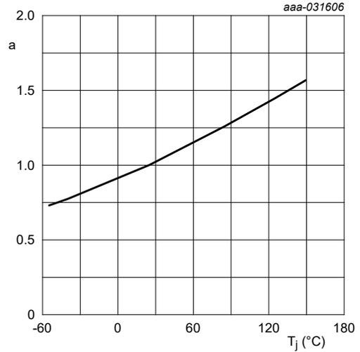
$$a = \frac{R_{DSon}}{R_{DSon(25^\circ\text{C})}}$$
