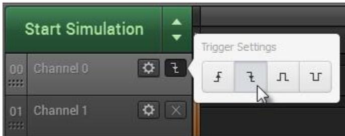
If desired, you can also require other channels to be either high or low during a previously selected edge. After selecting an edge, note that other channels will display a button with an "X" (indicates "don't care").
