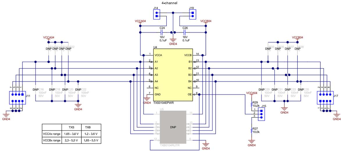
Figure 3-3. 4-Channel TXS0104E
