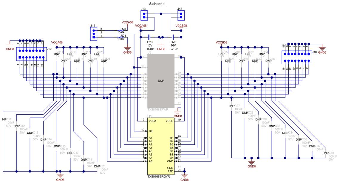
Figure 3-4. 8-Channel TXS0108E
