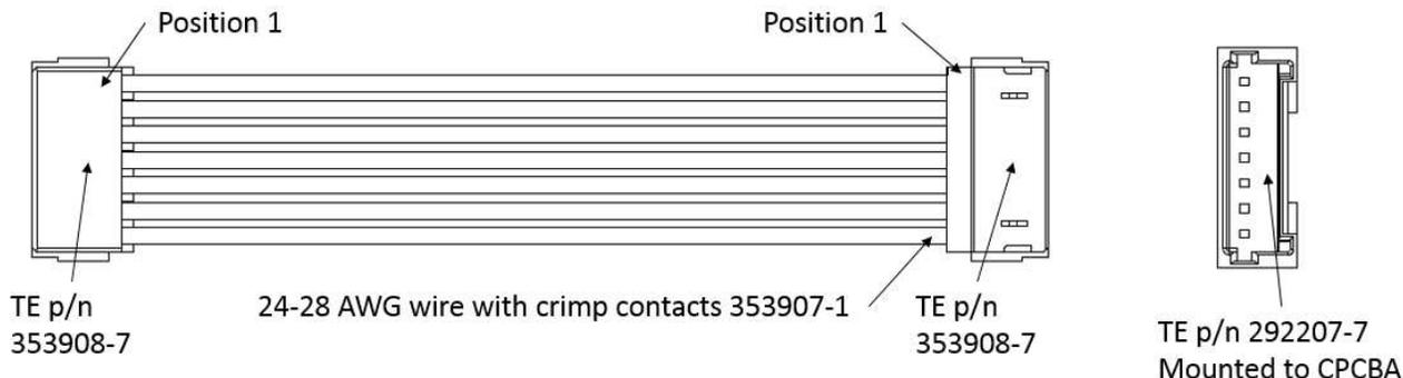
Figure 12. LCC Cable Assembly, TE p/n 2318043-1
