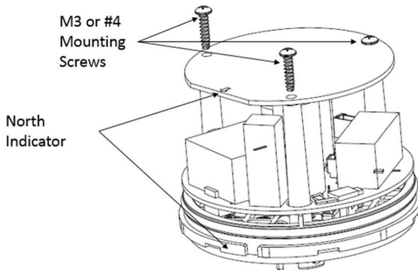
Figure 15. CPCBA Mounting
