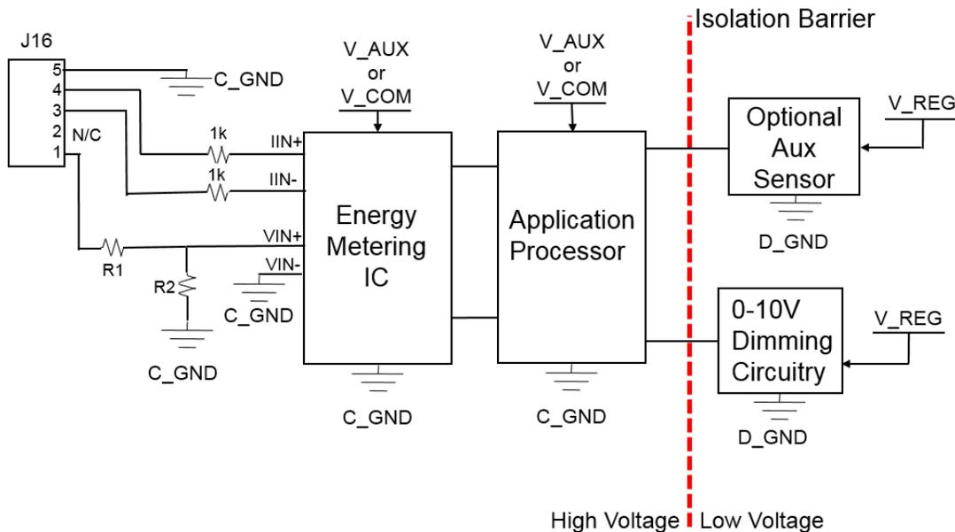
Figure 7. Energy Metering Implementation Architecture
