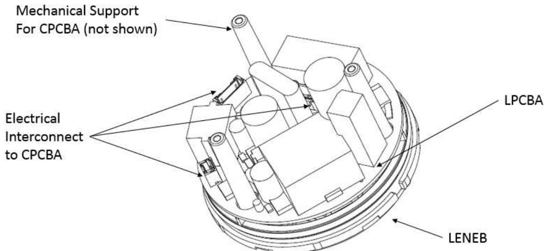
Figure 1. Control Node Layout using the LENE<sub>B</sub>
