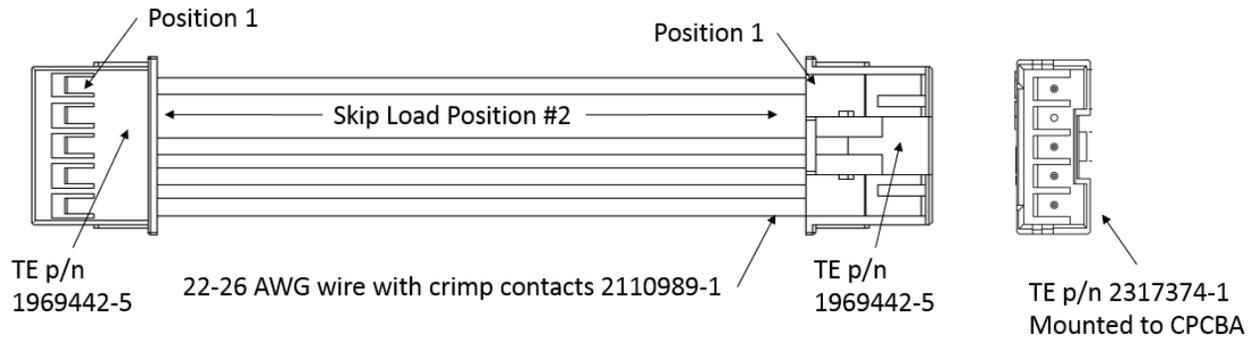
Figure 14. EMC Cable Assembly, TE p/n 2318044-1
