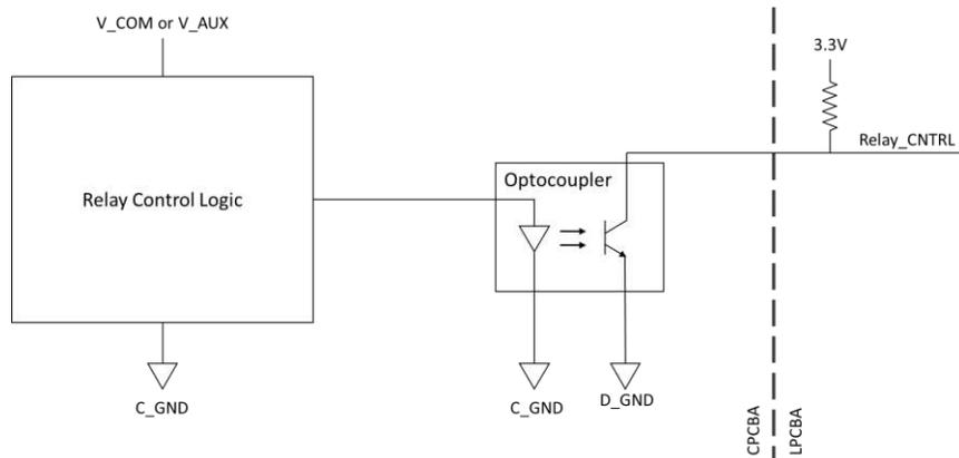
Figure 6. Relay Switching with Energy Metering (example)
