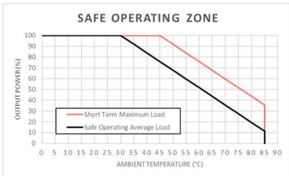
Figure 11 - Typical Application Derating Curve
