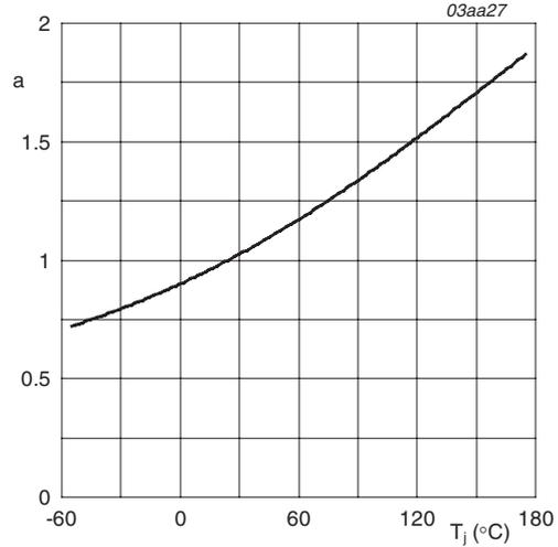
$$a = \frac{R_{DS(on)}}{R_{DS(on)(25^\circ\text{C})}}$$
