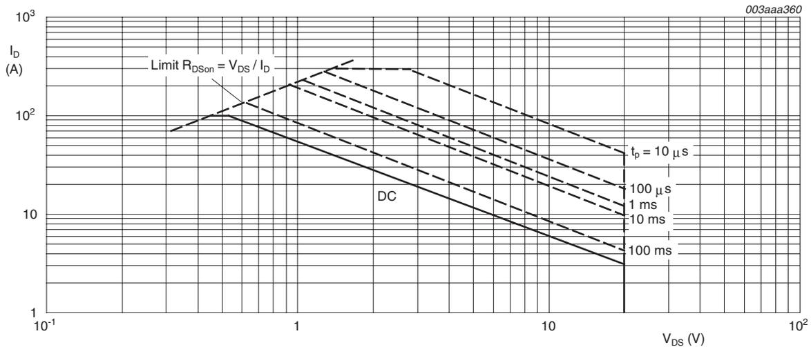
$T_{mb} = 25^\circ\text{C}; I_{DM}$  is single pulse;  $V_{GS} = 10\text{V}$
