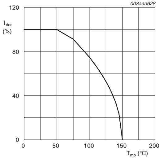
$$V_{GS} \geq 10 \text{ V}; I_{der} = \frac{I_D}{I_{D(25^\circ\text{C})}} \times 100 \%$$
