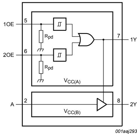
$R_{pd}$  = Internal pull-down resistor.
