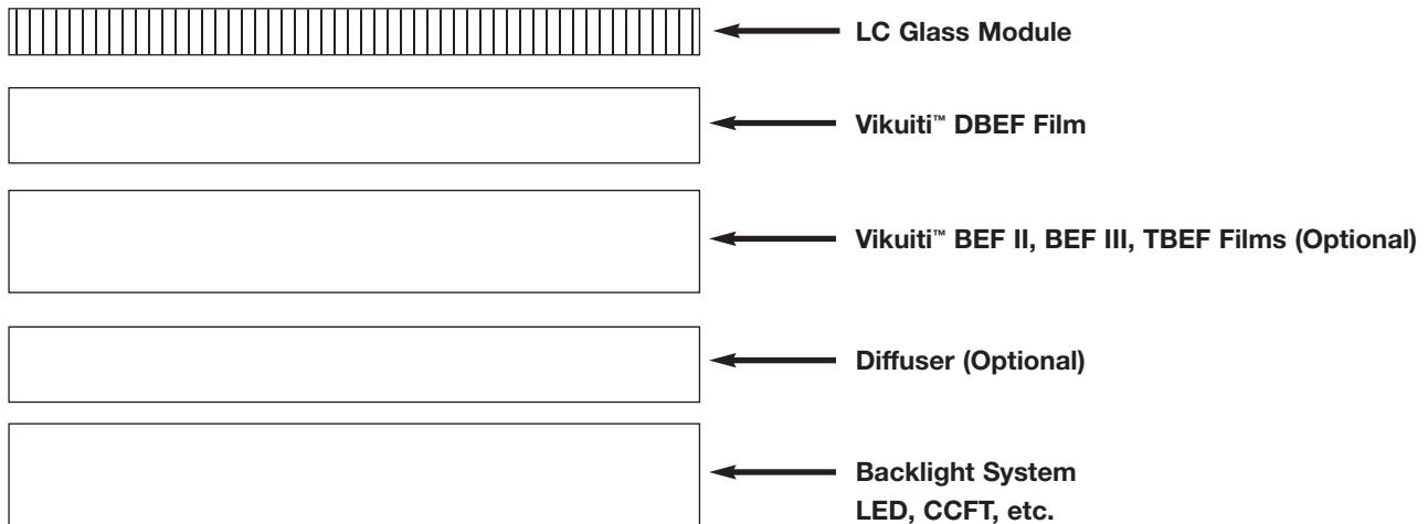
The film must be mounted with its transmission axis parallel to the transmission axis of the rear polarizer.
