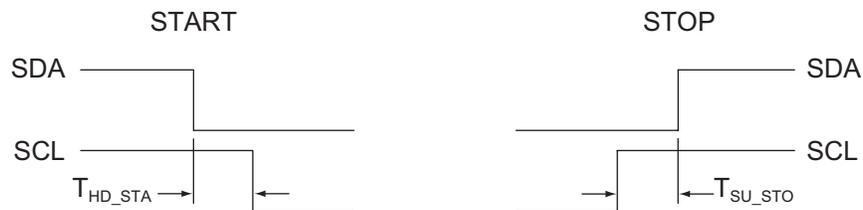
**Figure 2: I²C Start and Stop Conditions;**
