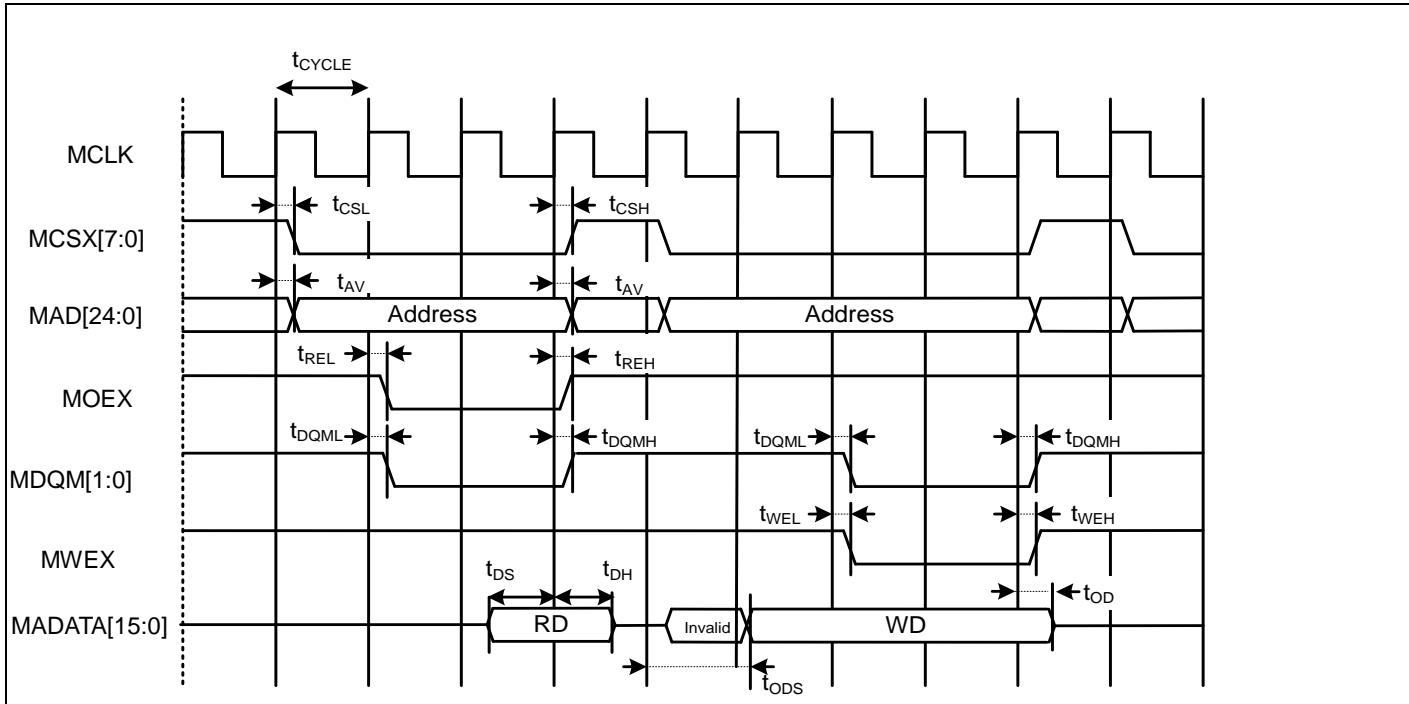
**Multiplexed Bus Access Asynchronous SRAM Mode**
