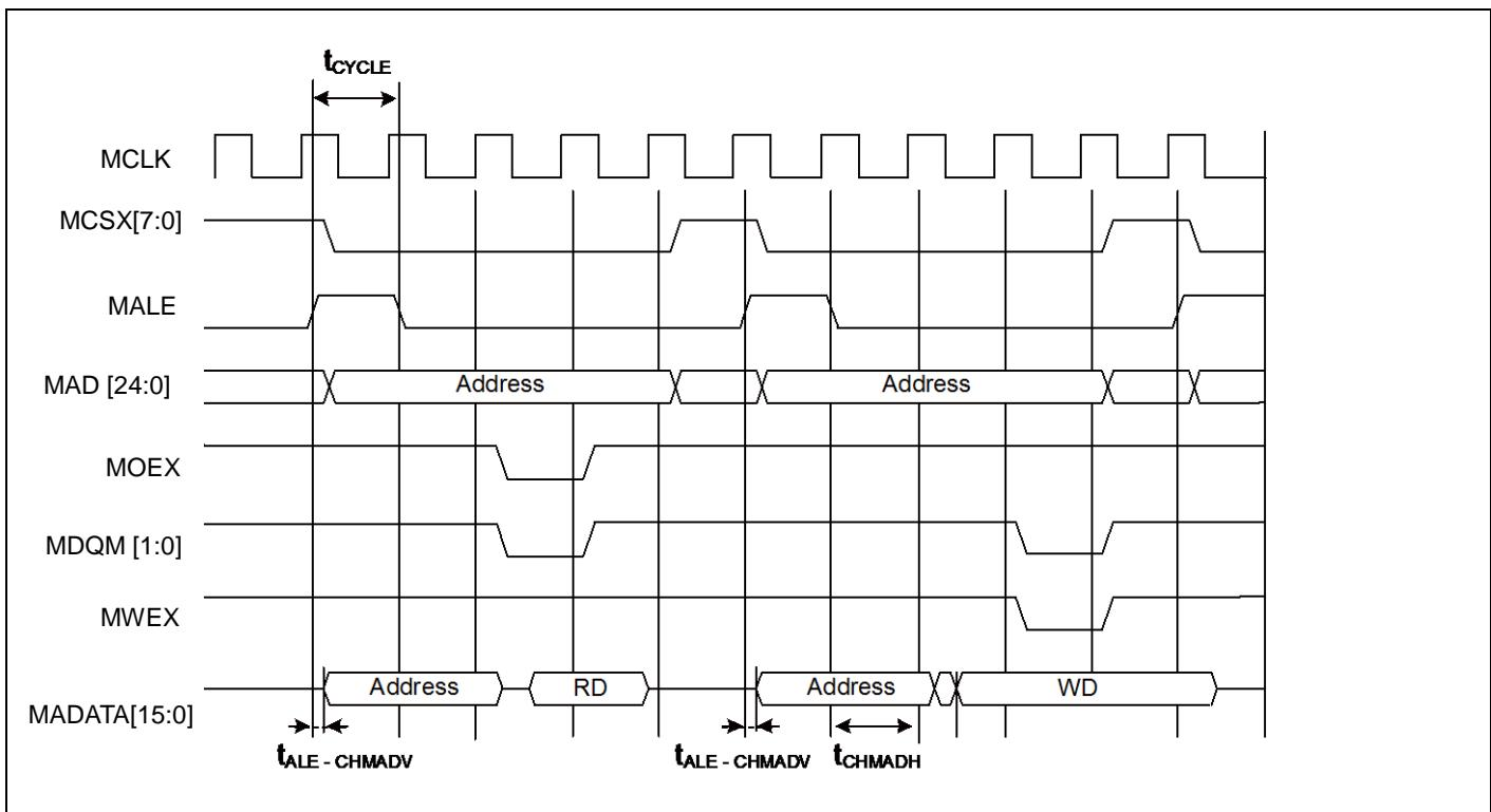
**Multiplexed Bus Access Synchronous SRAM Mode**
