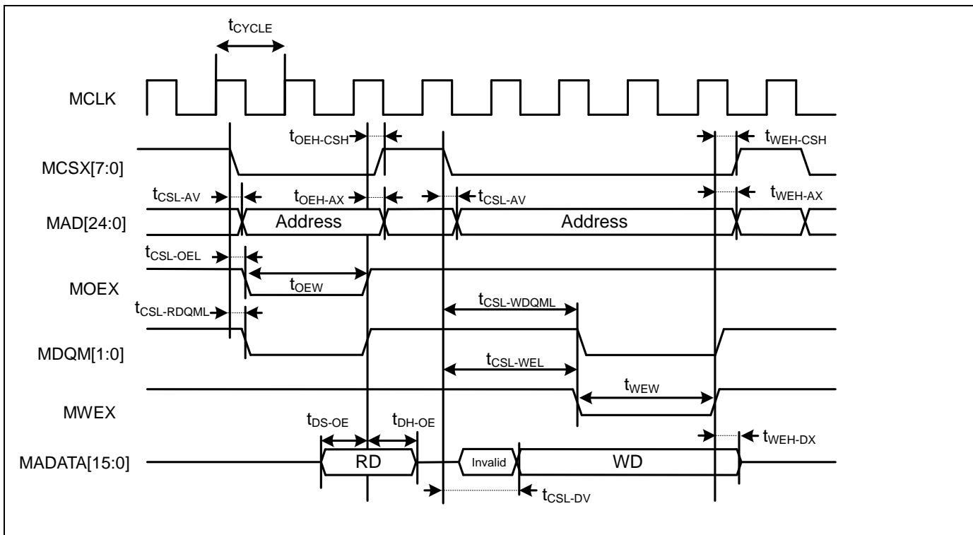
**Separate Bus Access Synchronous SRAM Mode**
