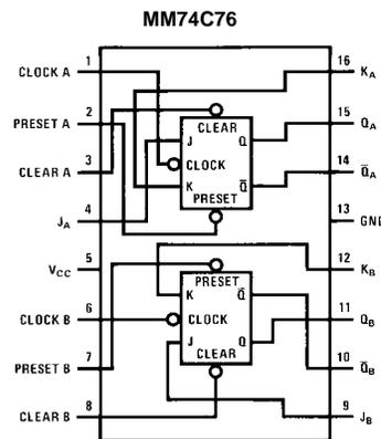
Note: A logic "0" on clear sets Q to a logic "0".
