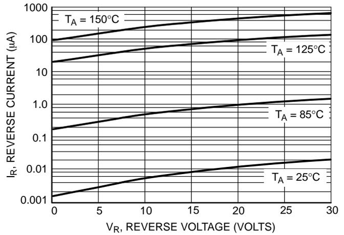
Figure 3. Leakage Current
