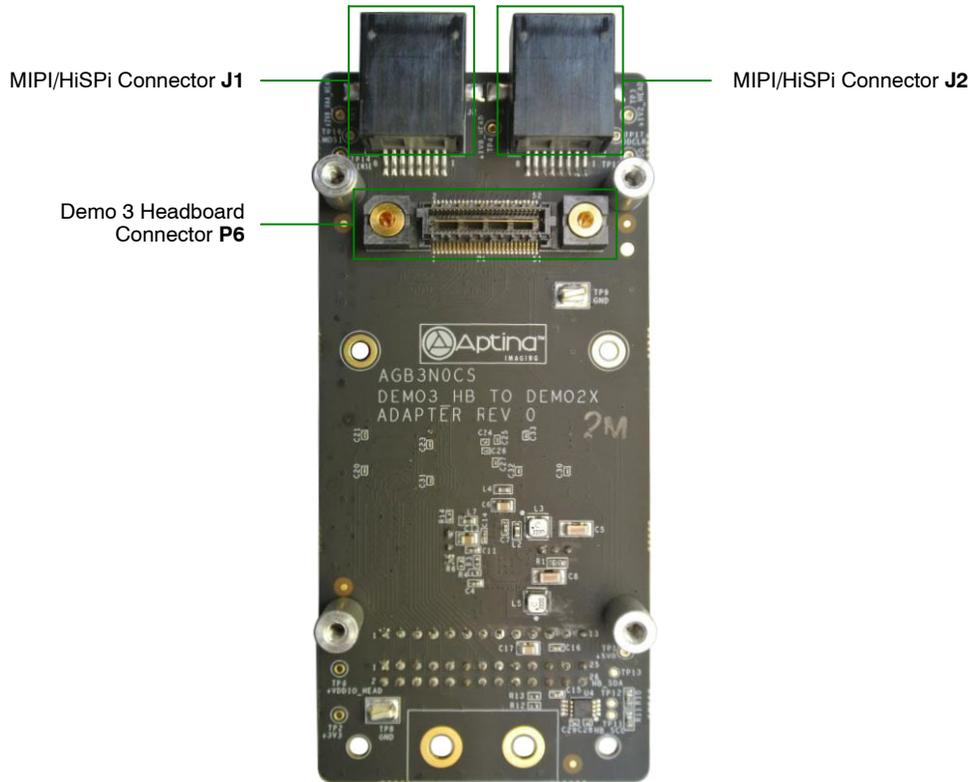
Figure 3. Top View of Adapter Board with Connectors
