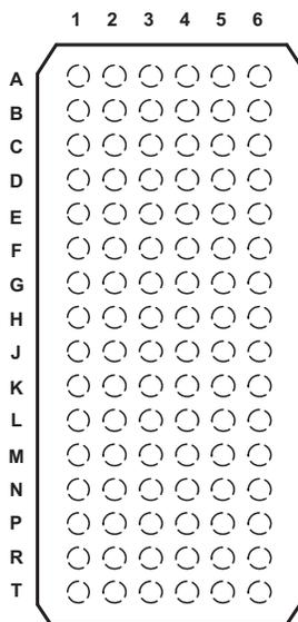
Figure 6-1. GKE, ZKE Package 96-Pin LFBGA Top View
