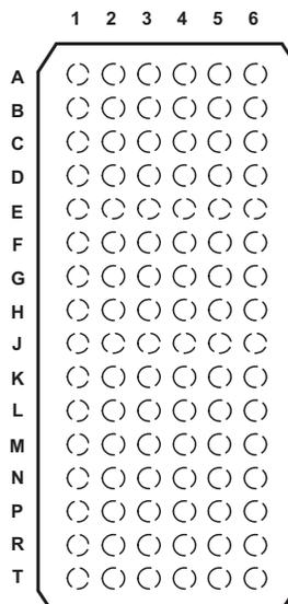
Figure 6-3. NMJ Package 96-Pin nFBGA Top View
