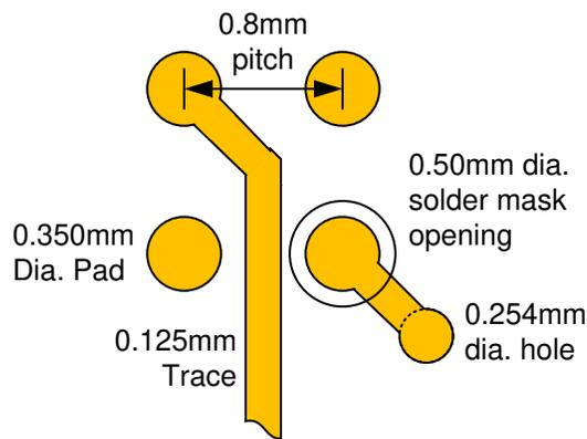
Figure 12-1. BGA Layout Example
