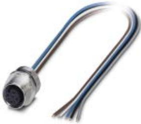
Sensor/Actuator flush-type socket, 5-pos., M12, A-coded, front/screw mounting with Pg9 thread, with 1 m TPE litz wire, 5x 0.34 mm<sup>2</sup>
