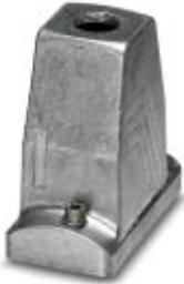
HEAVYCON ADVANCE sleeve housing B10, with high-grade steel screw locking (hexagonal socket-head), salt water resistant aluminum, height 100 mm, with thread, 1xM25, straight cable outlet, without surface; conductive seal (EMC properties)
