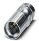
Cable connector, straight, Screw locking, M17, number of positions: 5+3+PE, type of contact: Socket, Crimp connection, shielded: yes, cable diameter range: 10 mm ... 12.5 mm
