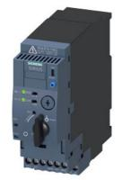
SIRIUS Compact load feeder DOL starter 690 V 24 V AC/DC 50...60 Hz 0.32...1.25 A IP20 Connection main circuit: plug-in, without terminals Connection auxiliary circuit: screw terminal
