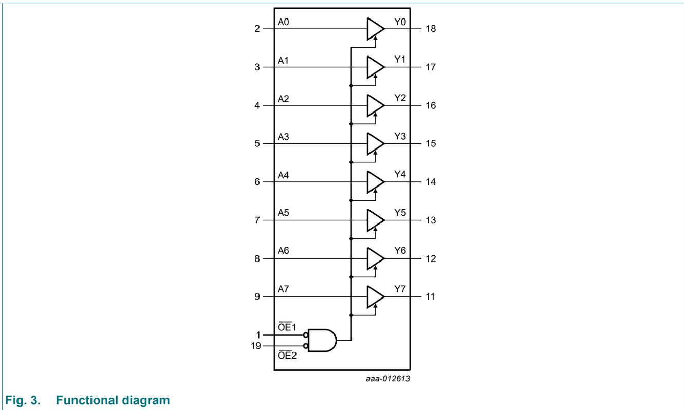
Fig. 3. Functional diagram
