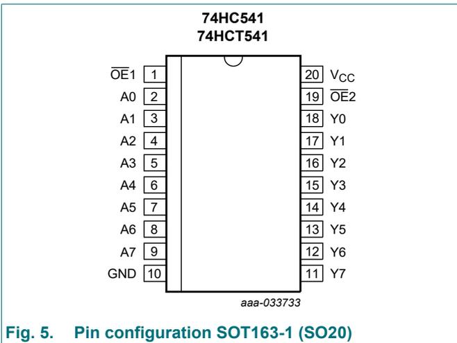
Fig. 5. Pin configuration SOT163-1 (SO20)
