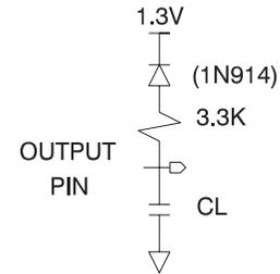
Note:  $C_L = 100 \text{ pF}$  including jig capacitance, except -45, -55, and -70 devices, where  $C_L = 30 \text{ pF}$ .
