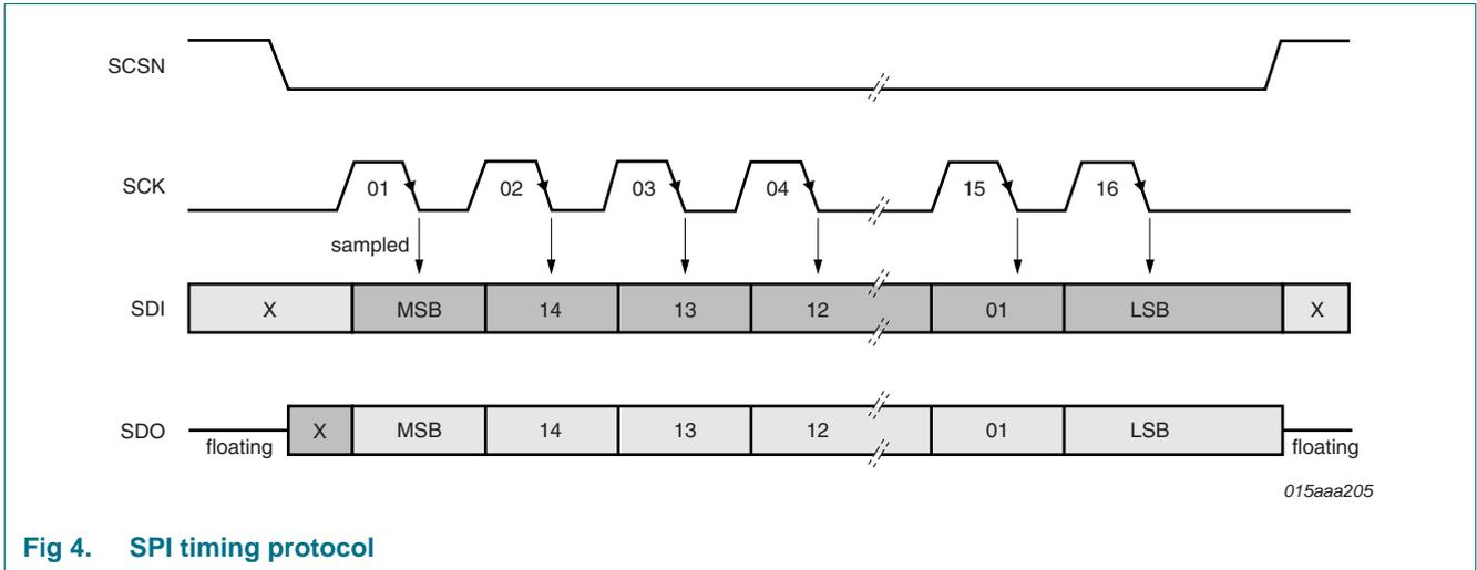
Fig 4. SPI timing protocol
