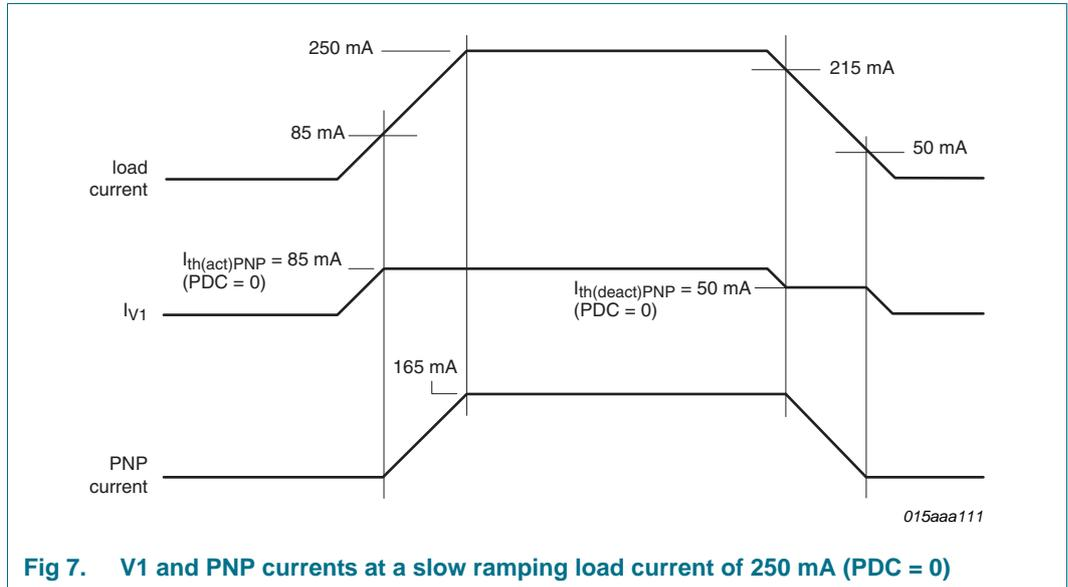
Figure 7 illustrates how V1 and the PNP transistor combine to supply a slow ramping load current of 250 mA with PDC = 0. Any additional load current requirement will be supplied by the PNP transistor, up to its current limit. If the load current continues to rise,  $I_{V1}$  will increase above the selected PDC threshold (to a maximum of 250 mA).
