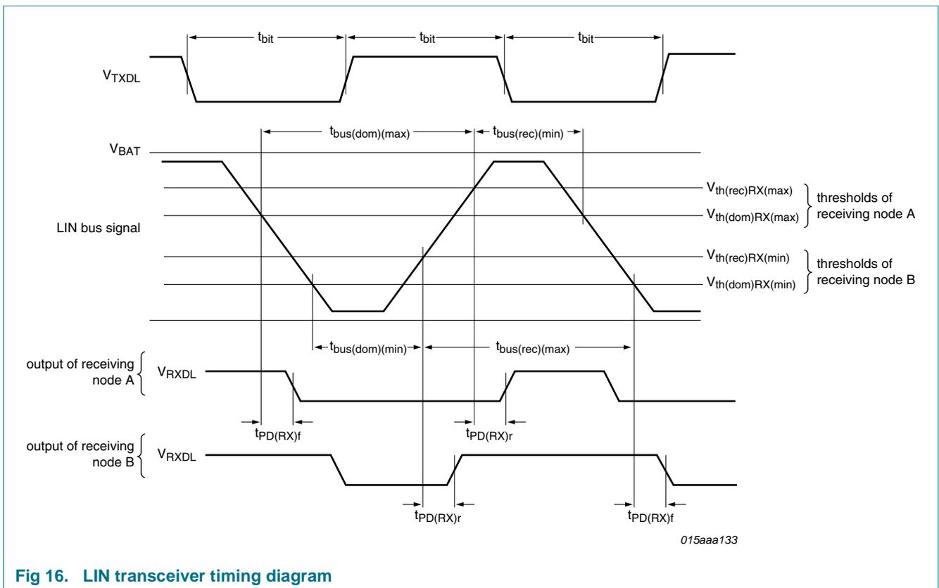
Fig 16. LIN transceiver timing diagram
