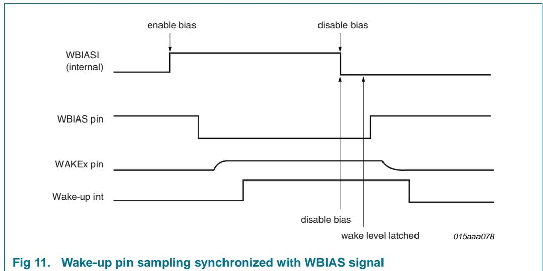
Fig 11. Wake-up pin sampling synchronized with WBIAS signal
