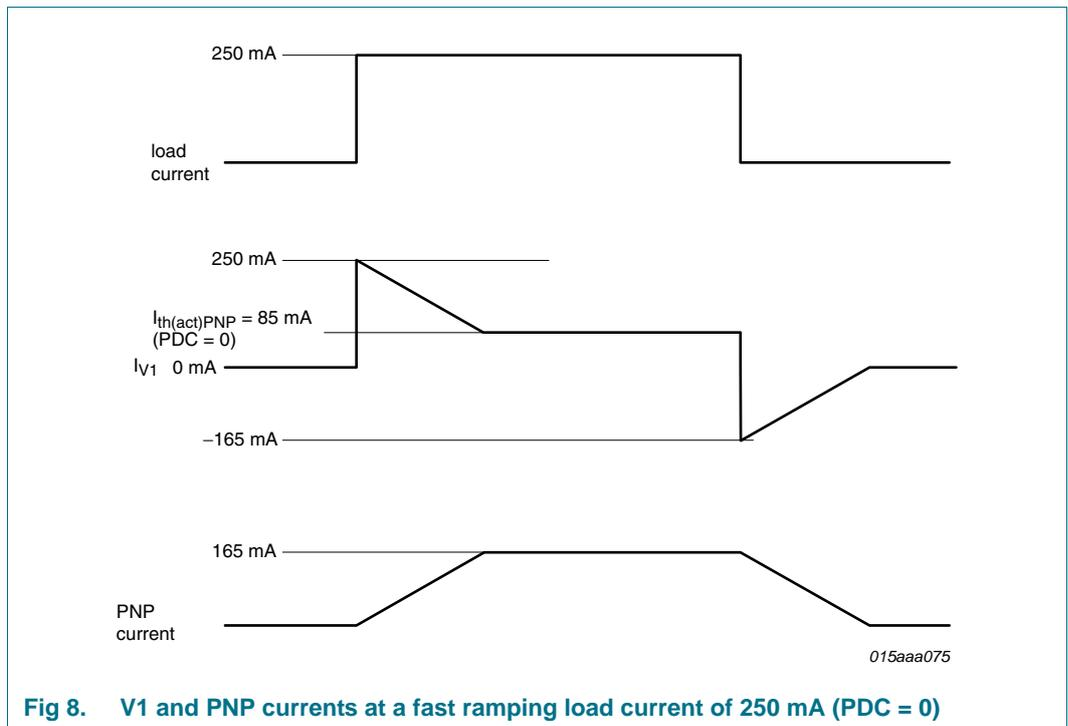
For short-circuit protection, a resistor needs to be connected between pins V1 and VEXCC to allow the current to be monitored. This resistor limits the current delivered by the external transistor. If the voltage difference between pins VEXCC and V1 reaches  $V_{th(act)lim}$ , the PNP current limiting activation threshold voltage, the transistor current will not increase further.
