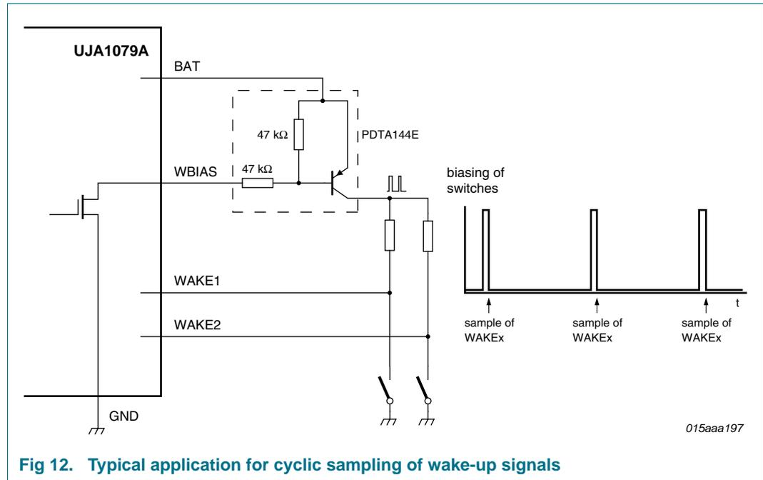
Fig 12. Typical application for cyclic sampling of wake-up signals
