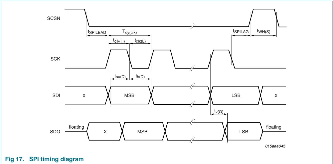
Fig 17. SPI timing diagram
