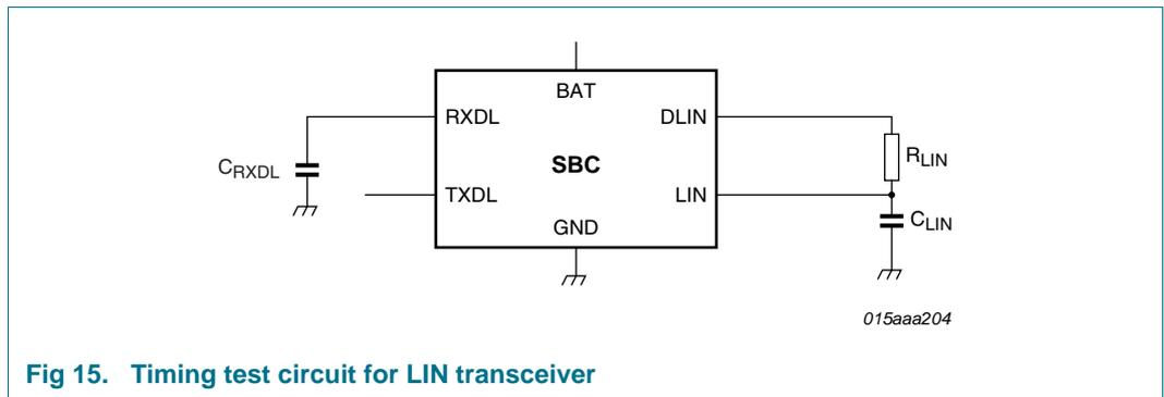
Fig 15. Timing test circuit for LIN transceiver
