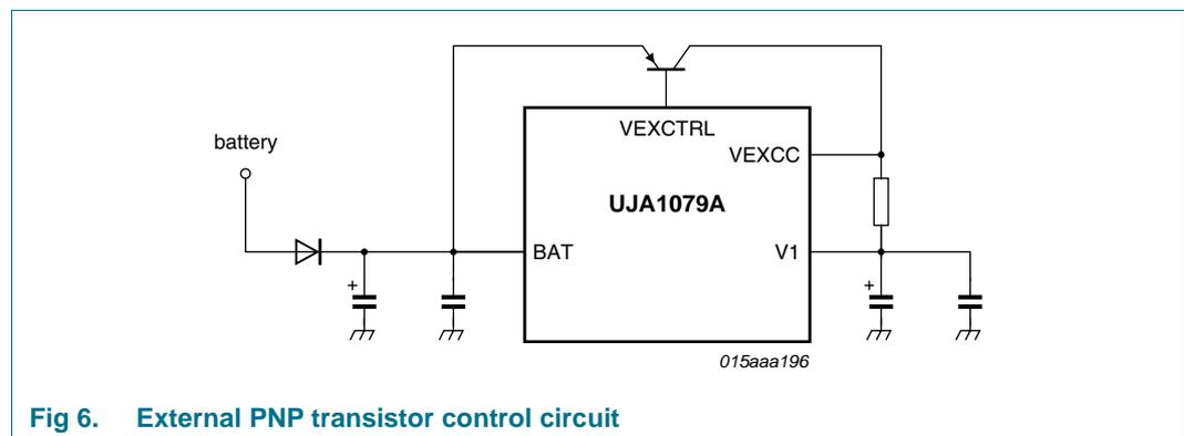
Fig 6. External PNP transistor control circuit
