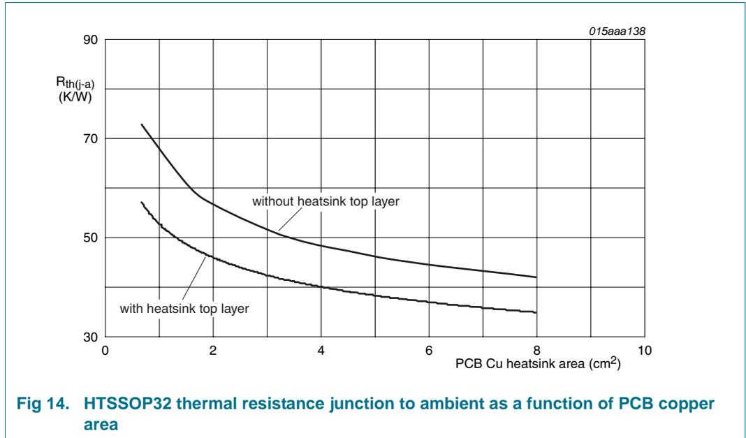
**Fig 14. HTSSOP32 thermal resistance junction to ambient as a function of PCB copper area**
