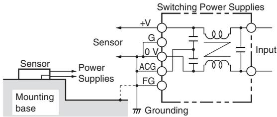
4. Insert a plastic insulator of approximately 10 mm between the Sensor and the mounting base.
