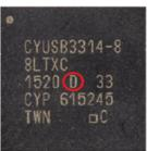
Cypress maintains traceability of product to wafer level, including wafer fabrication location, through the lot number marked on the package.
