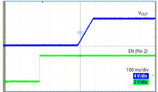
Figure 6: EN pin controlled turn on
