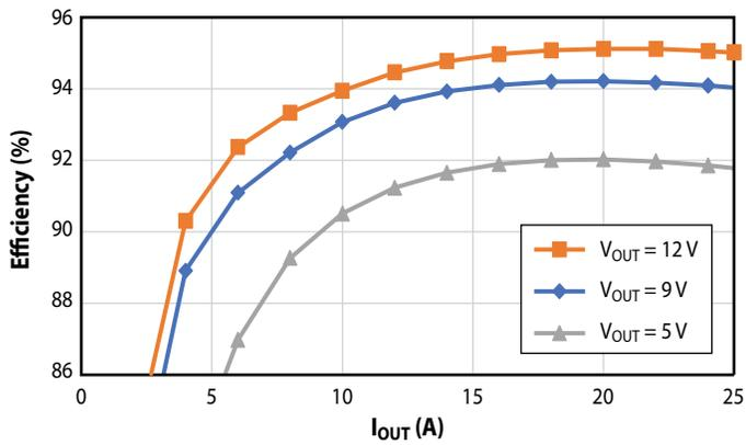
Figure 1: 48 V input, various output voltages
