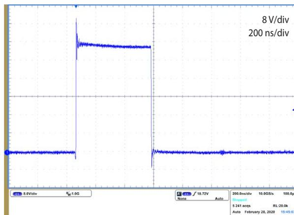
Figure 9: Measured switch-node voltage for one phase at  $V_{IN} = 48V, V_{OUT} = 12V, I_{OUT} = 25A$
