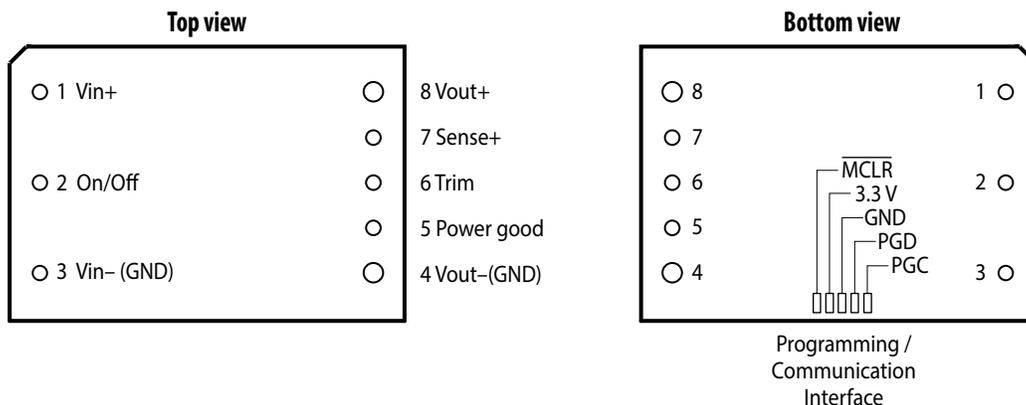
Figure 15: Pin assignment
