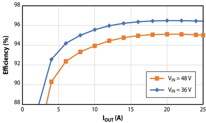
Figure 2: 12 V output, various input voltages
