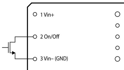
Figure 10. Adding an external MOSFET for remote enable/disable
