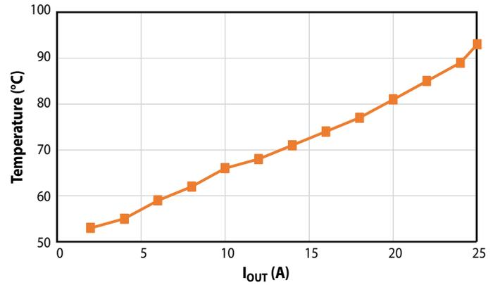
Figure 8:  $V_{IN} = 48V, V_{OUT} = 12V, 800\text{ LFM}$  forced air cooling
