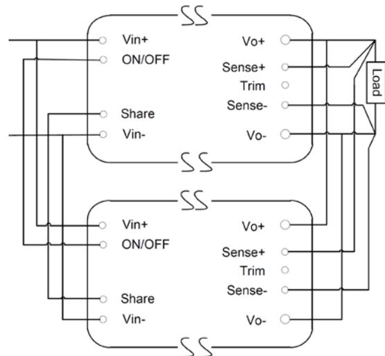
**Figure 15.** Circuit Configuration for Active Current Share
