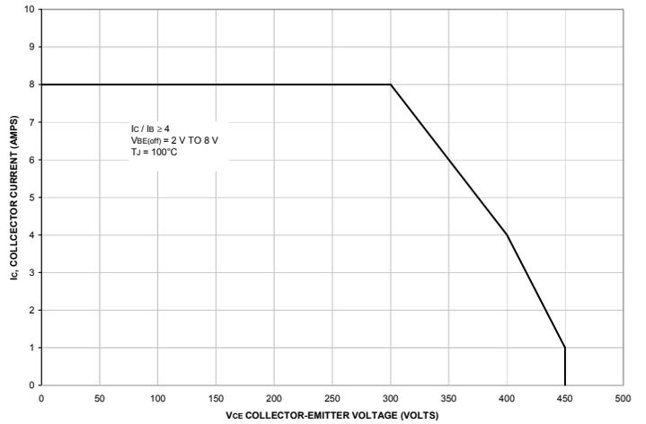
Figure 2. Reverse Bias Switching Safe Operating Area
