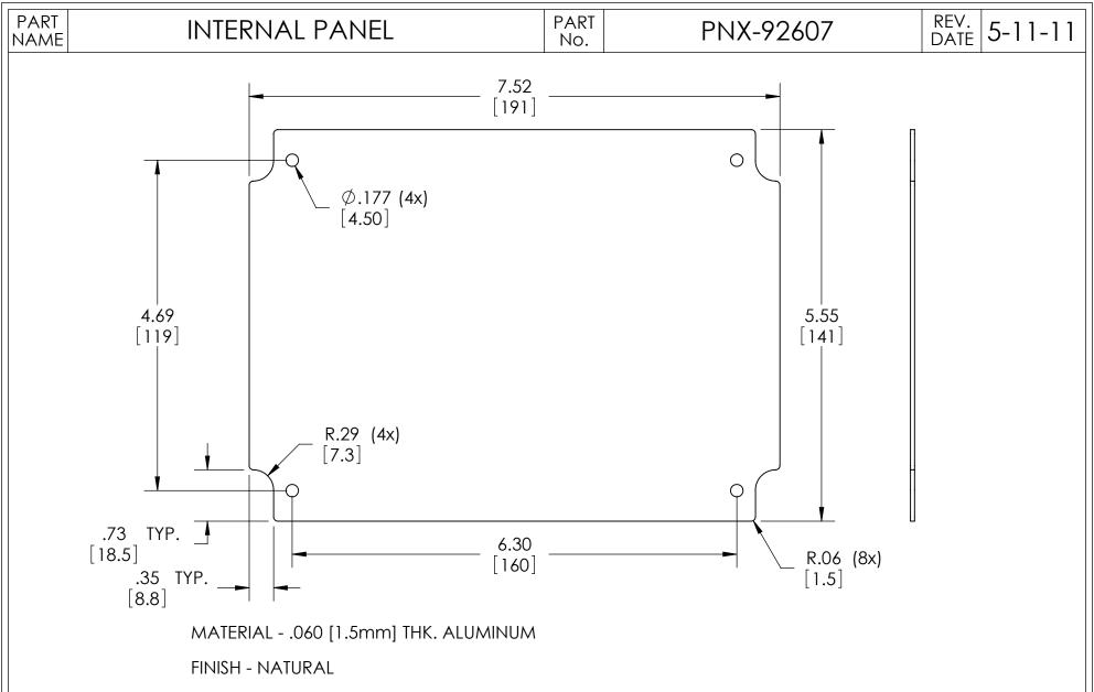
SUPPLIED WITH M3x0.5 x 6mm LG. MACHINE SCREWS (PAN HD., PHILLIPS DRIVE, STEEL, ZINC PLATED) FOR MOUNTING.
